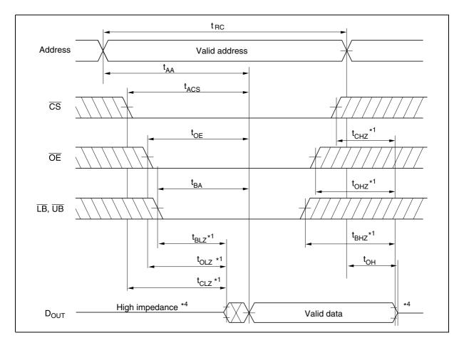
Read Timing Waveform (2)  $(\overline{WE}=V_{_{IH}},\overline{LB}=V_{_{IL}},\overline{UB}=V_{_{IL}})$
