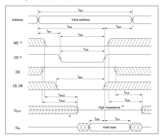
Write Timing Waveform (3) ( $\overline{LB}$ ,  $\overline{UB}$  Controlled,  $\overline{OE} = V_{HJ}$ )
