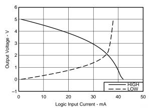
Figure 1. Output Voltage vs Input Current
