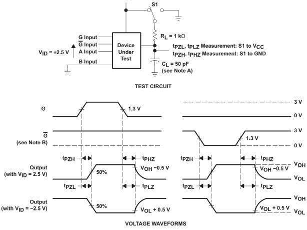
A. C<sub>L</sub> includes probe and jig capacitance.
