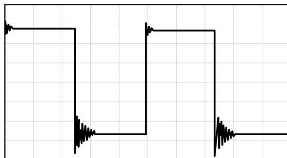
(b) C_L = 130 \text{ pF} , R_L = \text{NO LOAD}
