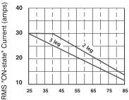
Ambient temperature (°C), measured 1 inch (25mm) below relay when mounted to DIN rail or a vertical, 1/8th inch thick aluminum panel surface. Airflow is unrestricted up and through the heat sink.
