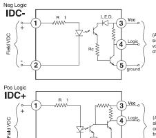
(A voltage on the field side will cause the voltage on terminal "4" to change from Vcc to ground)
