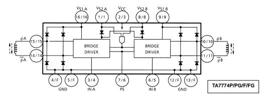
Note: Pins (2), (7), (12), (13) of TA7774F/FG are all NC, and the heat fin is connected to GND.
