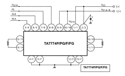
Note: Utmost care is necessary in the design of the output, V<sub>M</sub> and GND lines since the IC may be destroyed by short-circuiting between outputs, air contamination faults, or faults due to improper grounding.
