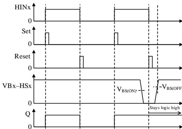
Figure 12-3. Waveforms at VB<sub>x</sub>–HS<sub>x</sub> Voltage Drop
