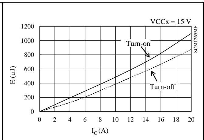
Figure 15-50. Low-side Switching Loss ( $T_J = 125\text{ }^\circ\text{C}$ )
