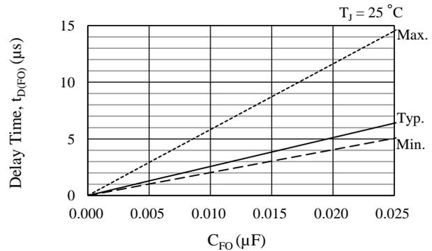
Figure 12-11. Delay Time,  $t_{D(FO)}$  vs. Filter Capacitor,  $C_{FO}$
