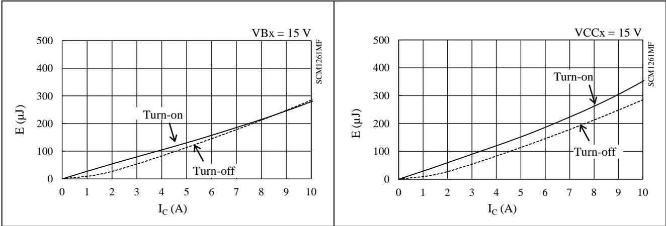
Figure 15-35. High-side Switching Loss ( $T_J = 25\text{ }^\circ\text{C}$ )
