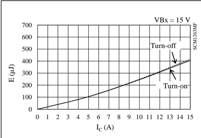
Figure 15-43 High-side Switching Loss ( $T_J = 25\text{ }^\circ\text{C}$ )
