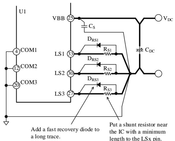
Figure 12-7. Connections to LS<sub>x</sub> Pin
