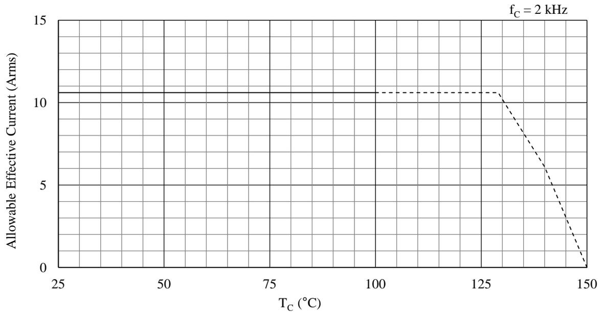
Figure 15-57. Allowable Effective Current ( $f_c = 2$  kHz): 15 A Devices
