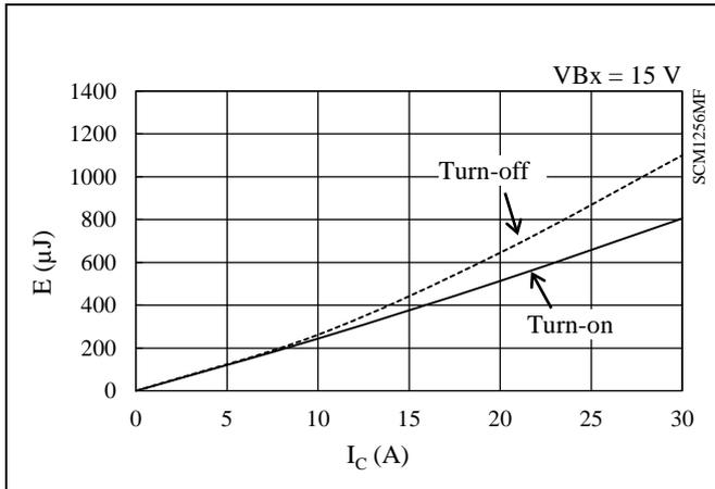
Figure 15-51. High-side Switching Loss ( $T_j = 25\text{ }^\circ\text{C}$ )
