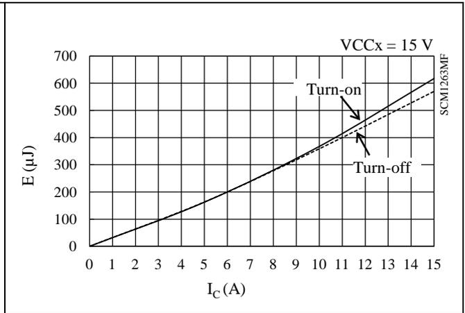
Figure 15-46. Low-side Switching Loss ( $T_J = 125\text{ }^\circ\text{C}$ )
