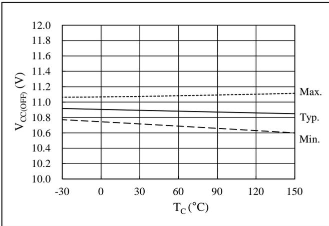
Figure 15-9. Logic Operation Stop Voltage,  $V_{CC(OFF)}$  vs.  $T_C$
