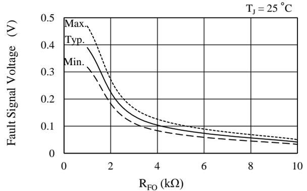
Figure 12-10. Fault Signal Voltage vs. Pull-up Resistor,  $R_{FO}$
