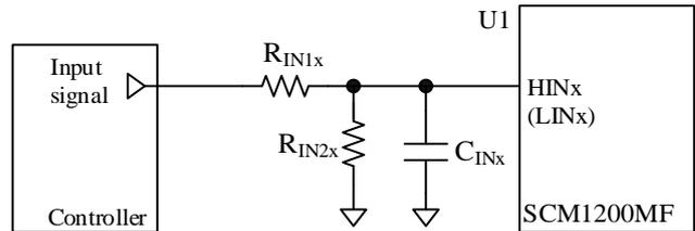
Figure 12-6. Filter Circuit for HIN<sub>x</sub> or LIN<sub>x</sub> Pin
