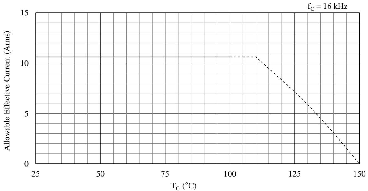
Figure 15-58. Allowable Effective Current ( $f_c = 16$  kHz): 15 A Devices
