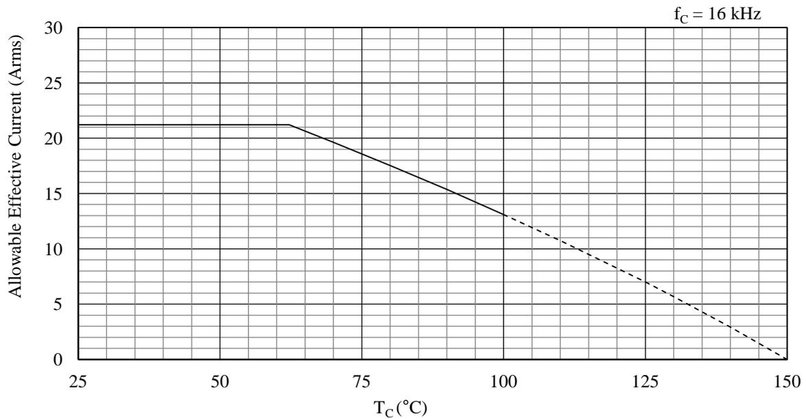
Figure 15-62. Allowable Effective Current ( $f_c = 16$  kHz): 30 A Devices
