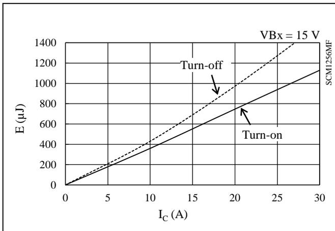
Figure 15-53. High-side Switching Loss ( $T_j = 125\text{ }^\circ\text{C}$ )
