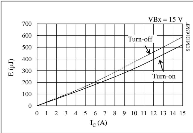
Figure 15-45. High-side Switching Loss ( $T_J = 125\text{ }^\circ\text{C}$ )
