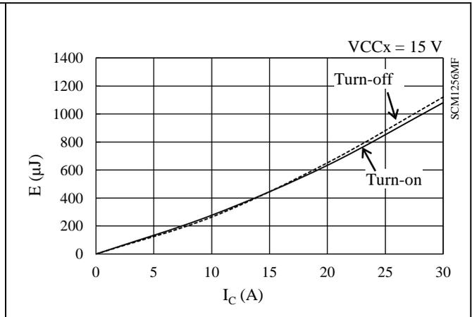
Figure 15-52. Low-side Switching Loss ( $T_j = 25\text{ }^\circ\text{C}$ )
