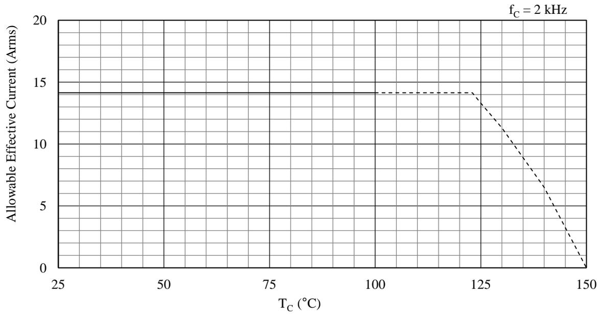
Figure 15-59. Allowable Effective Current ( $f_C = 2 \text{ kHz}$ ): 20 A Devices
