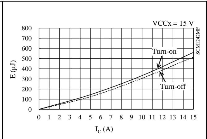
Figure 15-40. Low-side Switching Loss ( $T_J = 25\text{ }^\circ\text{C}$ )
