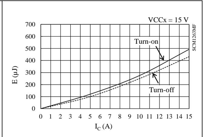
Figure 15-44. Low-side Switching Loss ( $T_J = 25\text{ }^\circ\text{C}$ )
