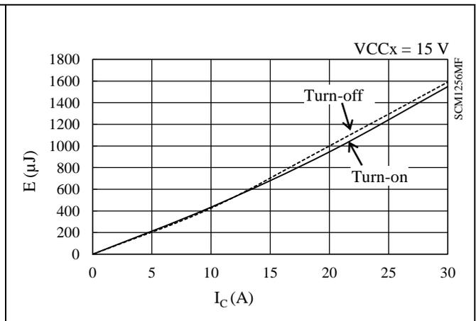
Figure 15-54. Low-side Switching Loss ( $T_j = 125\text{ }^\circ\text{C}$ )
