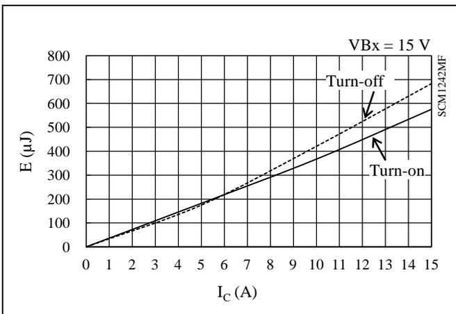
Figure 15-41. High-side Switching Loss ( $T_J = 125\text{ }^\circ\text{C}$ )
