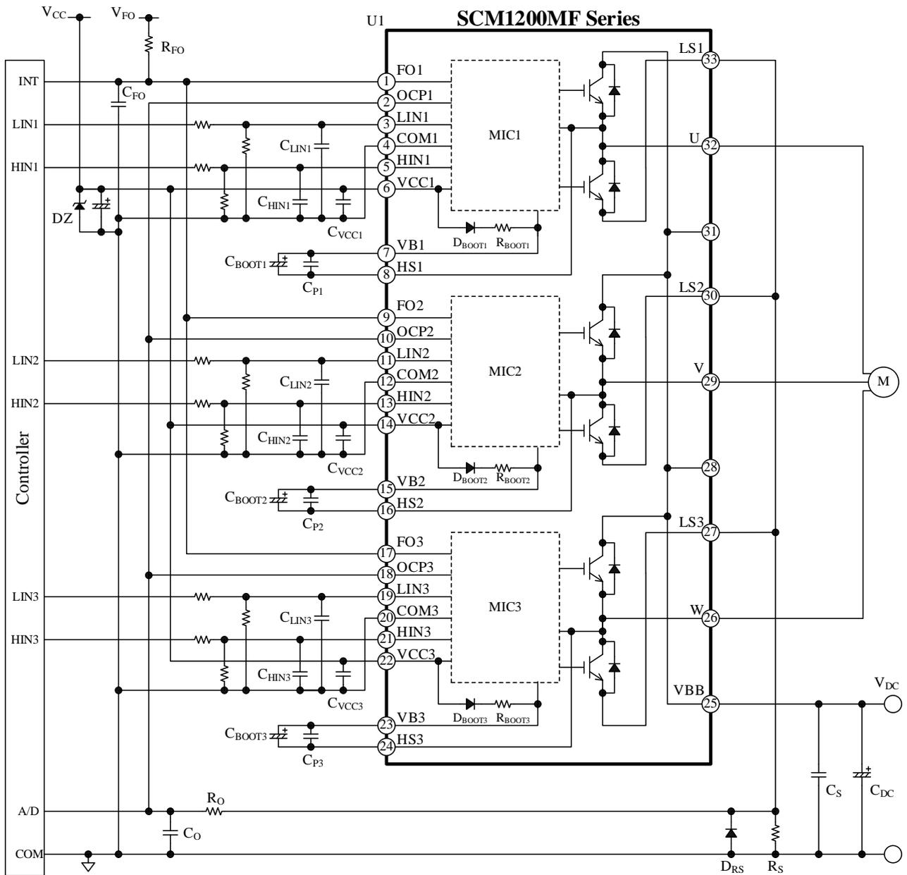
Figure 9-2. Typical Application Using a Single Shunt Resistor
