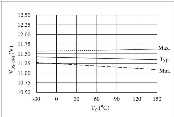
Figure 15-6. Logic Operation Start Voltage,  $V_{BS(ON)}$  vs.  $T_C$
