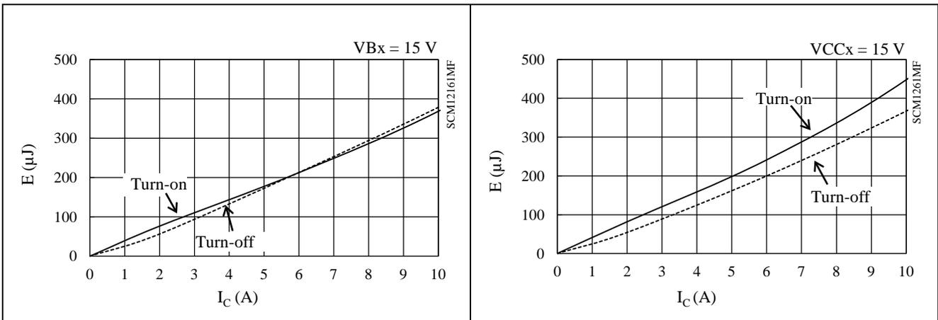
Figure 15-37. High-side Switching Loss ( $T_J = 125\text{ }^\circ\text{C}$ )
