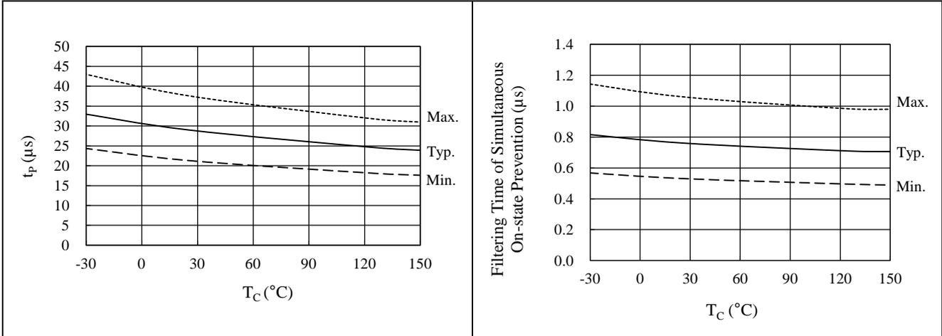
Figure 15-25. OCP Hold Time,  $t_p$  vs.  $T_C$
