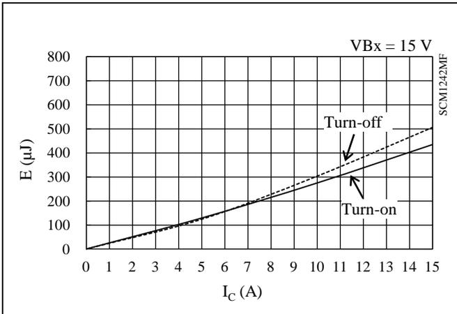
Figure 15-39 High-side Switching Loss ( $T_J = 25\text{ }^\circ\text{C}$ )
