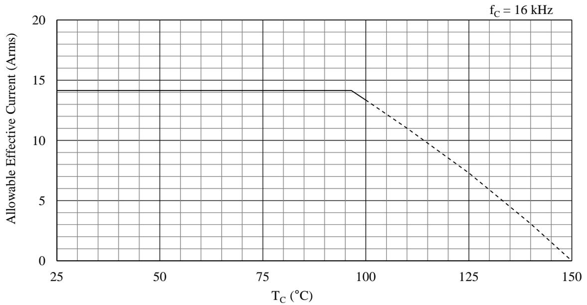
Figure 15-60. Allowable Effective Current ( $f_C = 16 \text{ kHz}$ ): 20 A Devices
