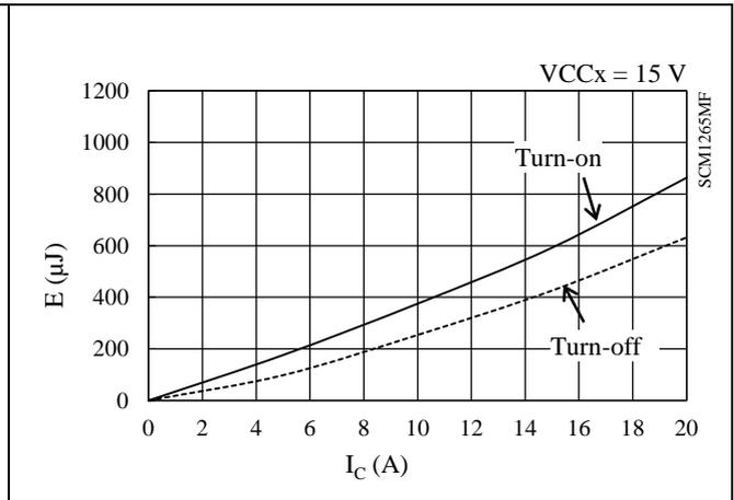
Figure 15-48. Low-side Switching Loss ( $T_J = 25\text{ }^\circ\text{C}$ )
