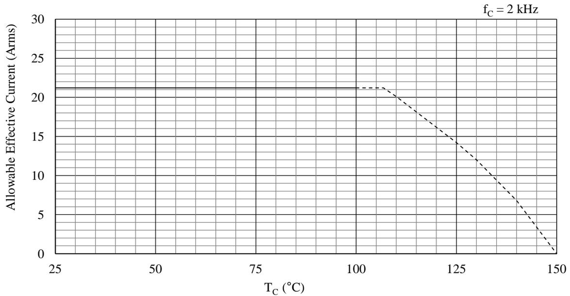
Figure 15-61. Allowable Effective Current ( $f_c = 2$  kHz): 30 A Devices
