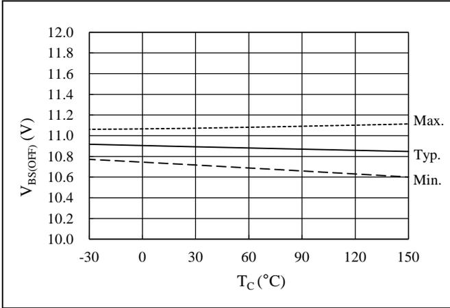
Figure 15-7. Logic Operation Stop Voltage,  $V_{BS(OFF)}$  vs.  $T_C$
