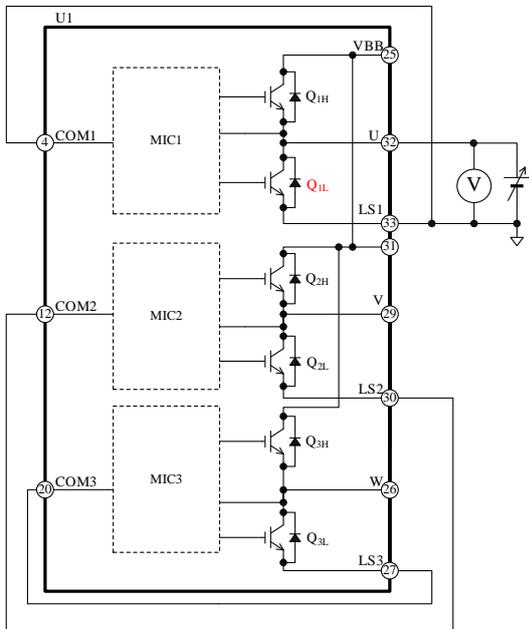
Figure 13-4. Typical Measurement Circuit for Low-side Transistor (Q<sub>1L</sub>) in U-phase
