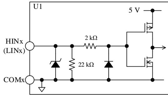
Figure 12-5. Internal Circuit Diagram of HIN<sub>x</sub> or LIN<sub>x</sub> Pin
