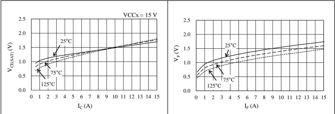
Figure 15-29. IGBT  $V_{CE(SAT)}$  vs.  $I_C$
