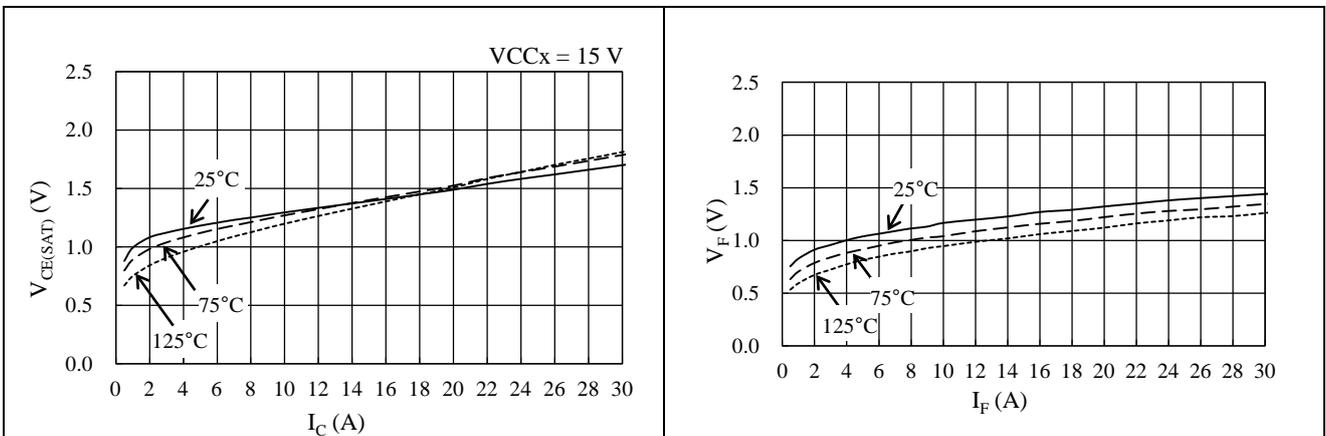
Figure 15-33. IGBT  $V_{CE(SAT)}$  vs.  $I_C$
