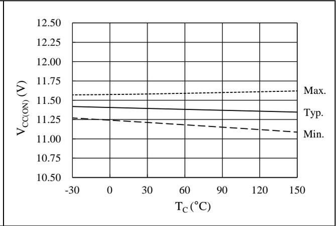
Figure 15-8. Logic Operation Start Voltage,  $V_{CC(ON)}$  vs.  $T_C$
