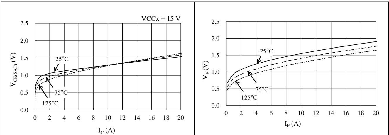
Figure 15-31. IGBT  $V_{CE(SAT)}$  vs.  $I_C$
