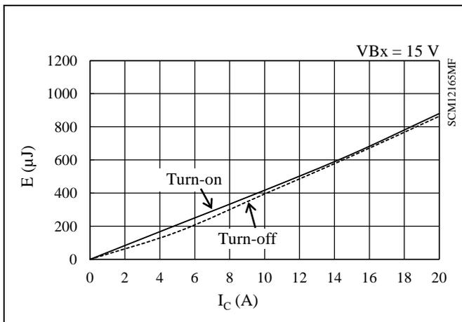
Figure 15-49. High-side Switching Loss ( $T_J = 125\text{ }^\circ\text{C}$ )
