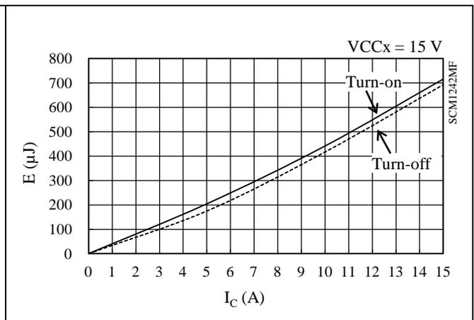
Figure 15-42. Low-side Switching Loss ( $T_J = 125\text{ }^\circ\text{C}$ )
