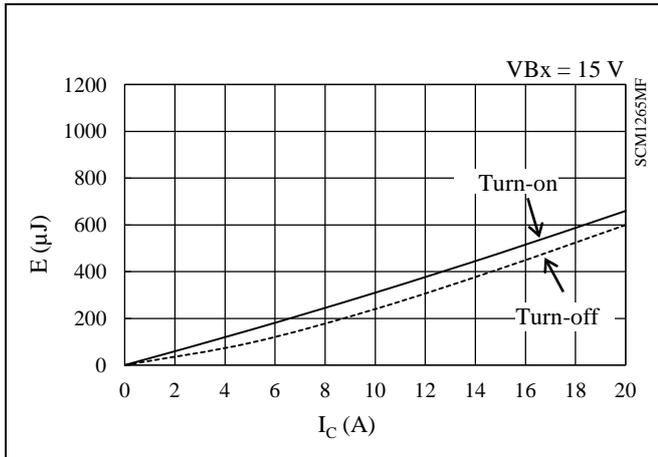
Figure 15-47 High-side Switching Loss ( $T_J = 25\text{ }^\circ\text{C}$ )
