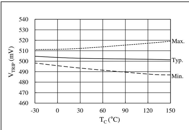
Figure 15-23. OCP Threshold Voltage,  $V_{TRIP}$  vs.  $T_C$
