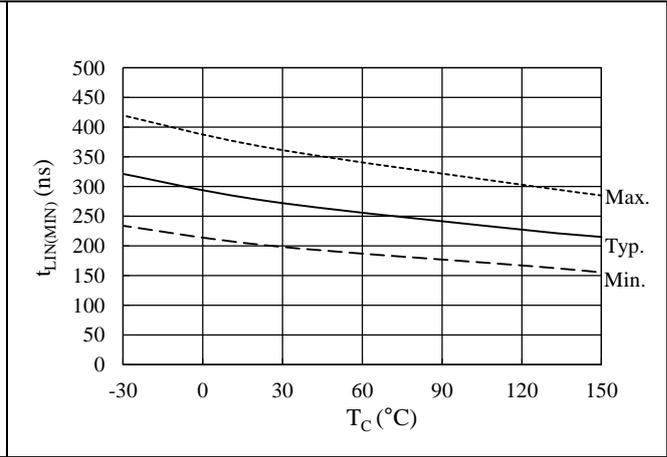
Figure 15-20. Minimum Transmittable Pulse Width for Low-side Switching,  $t_{LIN(MIN)}$  vs.  $T_C$
