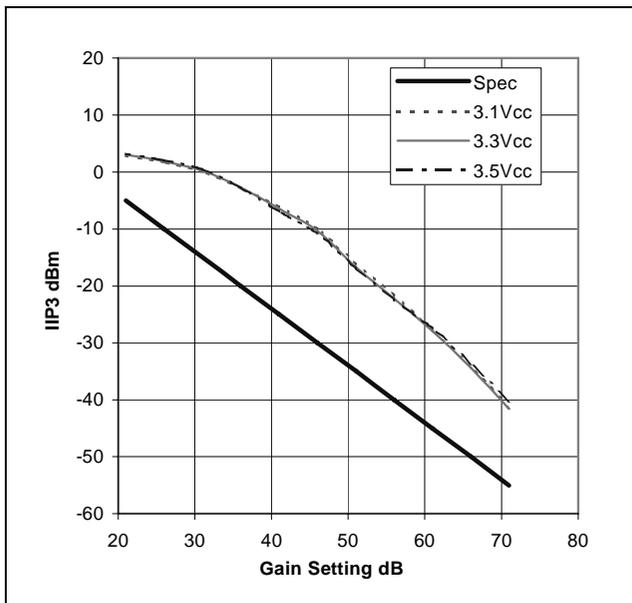
Figure 7 - IIP3 v Gain at 25°C
