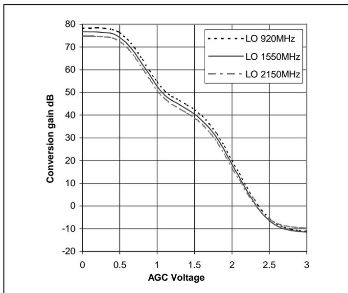
Figure 5 - Gain v. RFAGC at 25°C
