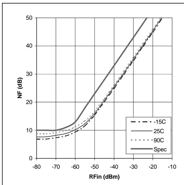
Figure 12 - Noise Figure v RFin v Temperature
