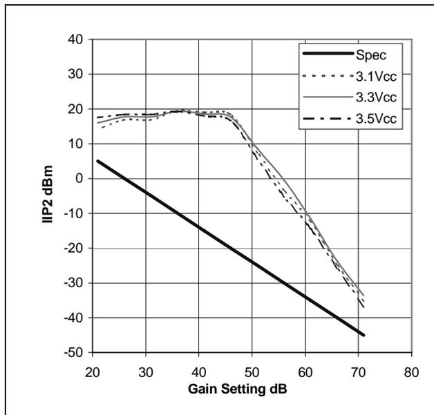
Figure 9 - IIP2 v Gain at 25°C
