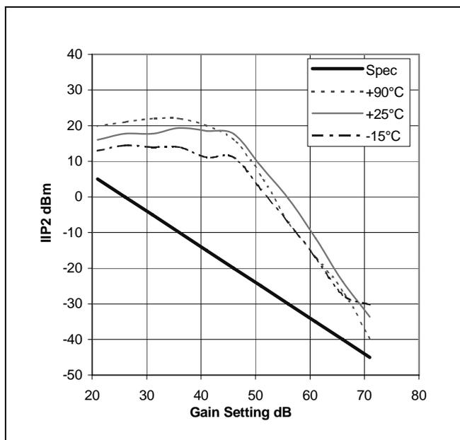
Figure 10 - IIP2 v Gain v Temperature
