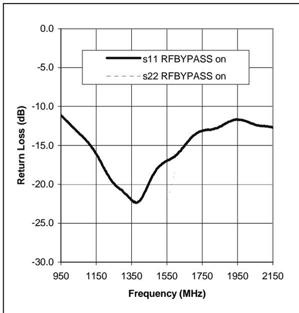
Figure 15 - RFin, RF Bypass Return Loss
