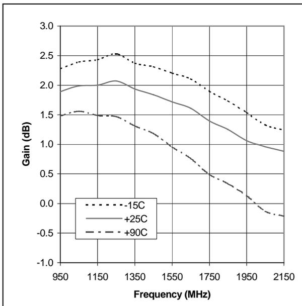
Figure 16 - RF Bypass Gain v Temperature
