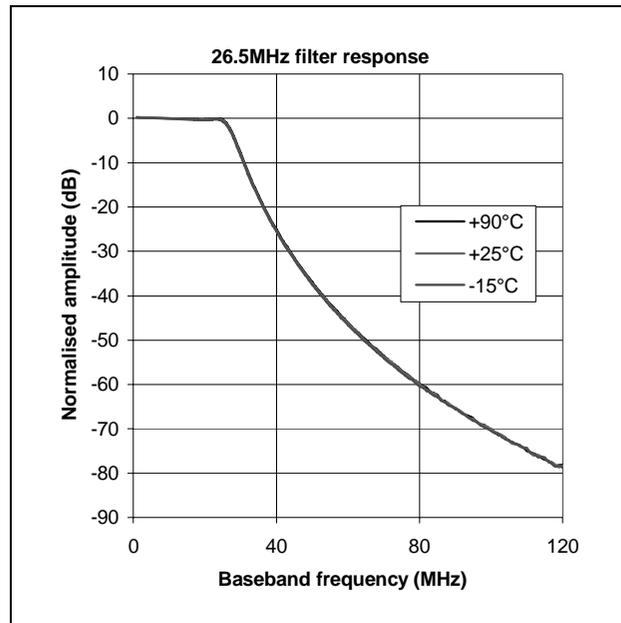
Figure 17 - Baseband Filter Response 26.5 MHz
