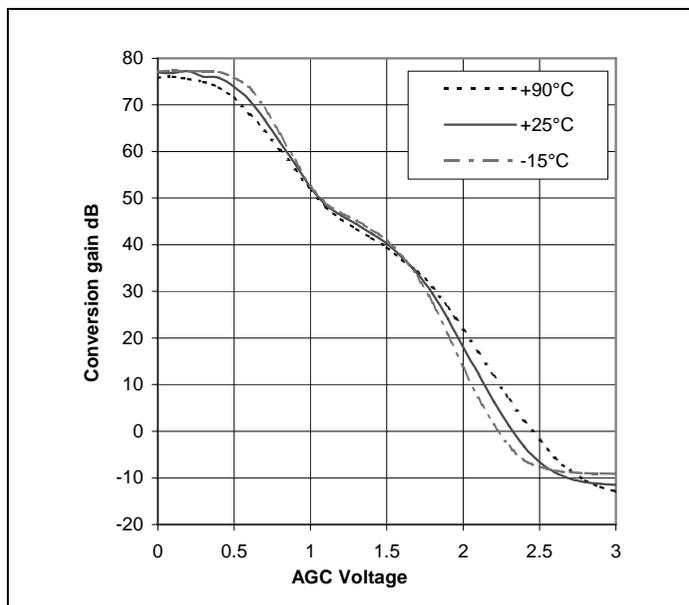
Figure 6 - Gain v RFAGC v. Temperature
