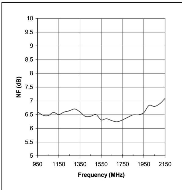
Figure 11 - Noise Figure v Freq at 25°C
