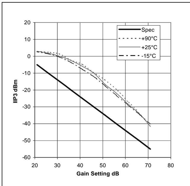
Figure 8 - IIP3 v Gain v Temperature
