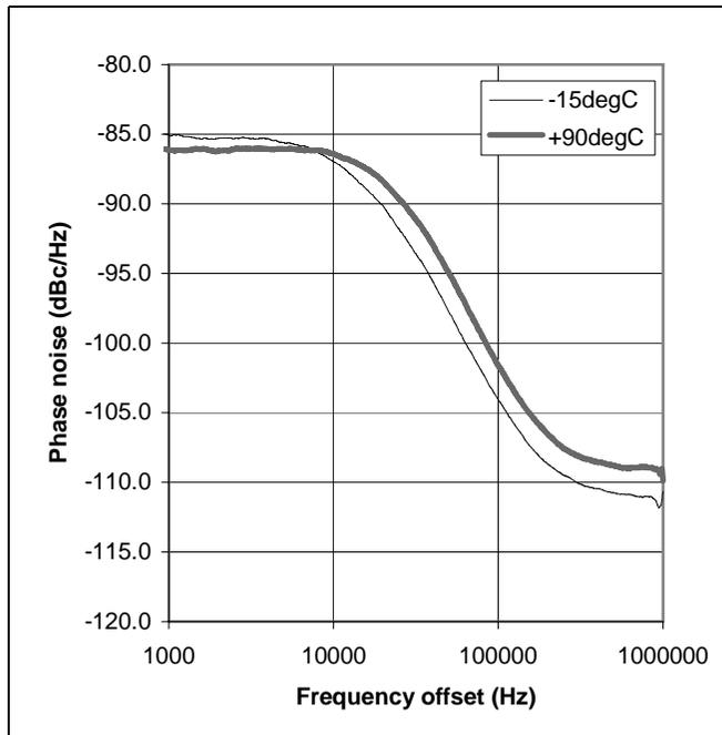
Figure 14 - LO Phase Noise v Temperature
