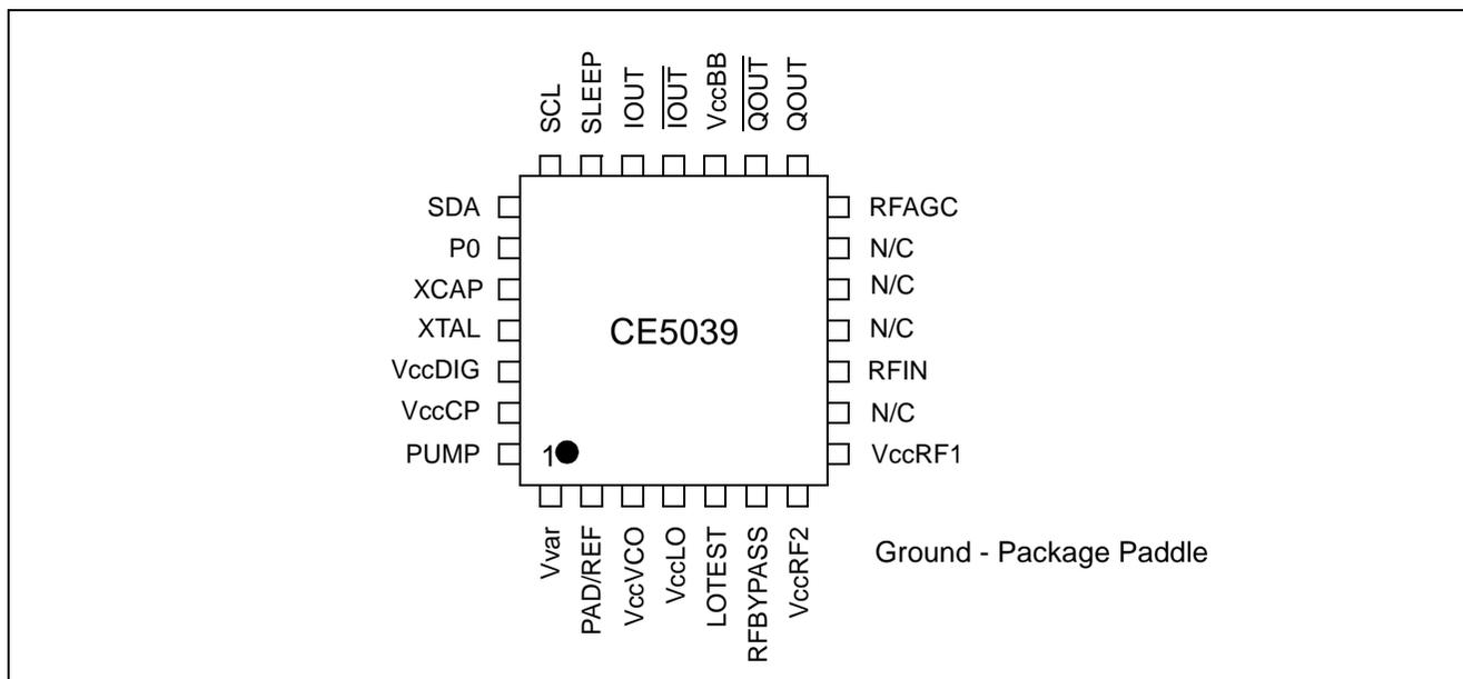
Figure 2 - Pin Diagram
