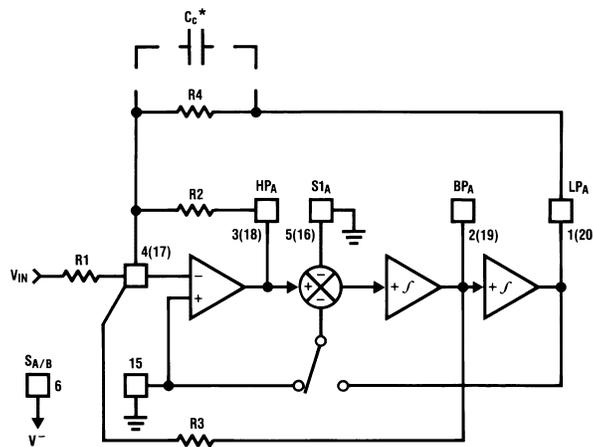
\*In Mode 3, the feedback loop is closed around the input summing amplifier; the finite GBW product of this op amp causes a slight Q enhancement. If this is a problem, connect a small capacitor (10 pF – 100 pF) across R4 to provide some phase lead.
