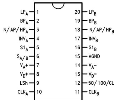
**Figure 38. SOIC and PDIP Packages (Top View)
