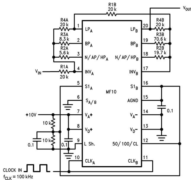
**Figure 33. Fourth-Order Chebyshev Low-Pass Filter from Example in 3.1. Single +10V Power Supply. 0V–5V TTL Logic Levels. Input Signals Should be Referred to Half-Supply or Applied through a Coupling Capacitor.**
