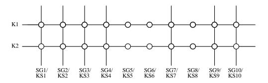
Each data entered by each key is stored as follows and read by a READ Command, starting from the last significant bit. When the most significant bit of the data (b0) has been read, the least significant bit of the next data (b7) is read.
