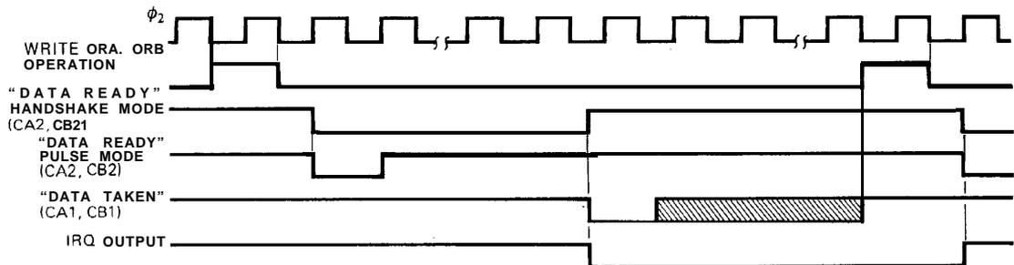
Figure 13. Write Handshake Timing
