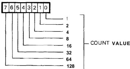
**WRITE** – 8 BITS LOADED INTO T2 LOW-ORDER LATCHES.
