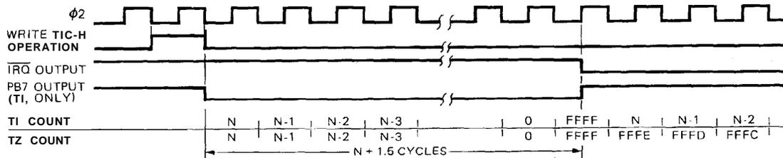
Figure 18. Timer 1 and Timer 2 One-Shot Mode Timing
