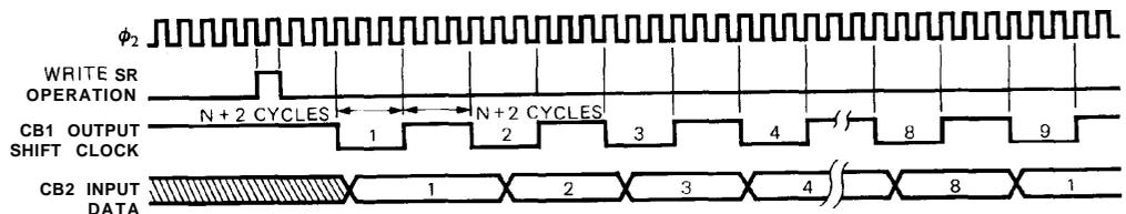
**Figure 24-1 Shift Register Output Modes**
