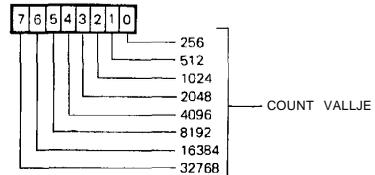
WRITE - 8 BITS LOADED INTO T1 HIGH-ORDER LATCHES. UNLIKE REG. 4 OPERATION, NO LATCH-TO-COUNTER TRANSFERS TAKE PLACE.
