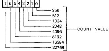
WRITE - 6 BITS LOADED INTO T1 HIGH-ORDER LATCHES. ALSO, AT THIS TIME BOTH HIGH AND LOW-ORDER LATCHES ARE TRANSFERRED INTO THE T1 COUNTER, AND INITIATES COUNTDOWN. T1 INTERRUPT FLAG IS ALSO RESET.
