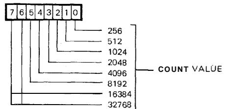
**WRITE** – 8 BITS LOADED INTO T2 HIGH-ORDER COUNTER. ALSO, LOW-ORDER LATCHES TRANSFERRED TO LOW-ORDER COUNTER. IN ADDITION, T2 INTERRUPT FLAG IS RESET.
