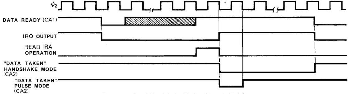
Figure 12. Read Handshake Timing (Port A, Only)
