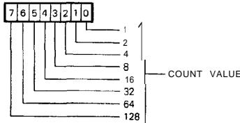
WRITE - 8 BITS ARE LOADED INTO T1 LOW-ORDER LATCHES. THIS OPERATION IS NO DIFFERENT FOLLOWING A WRITE INTO REG. 4.
