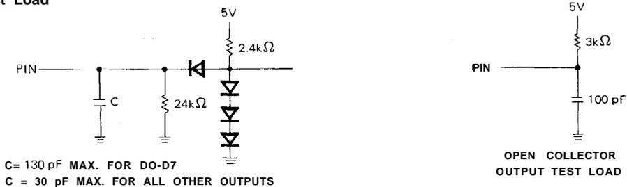
**Figure 2. Test Load (for all Dynamic Parameters)**
