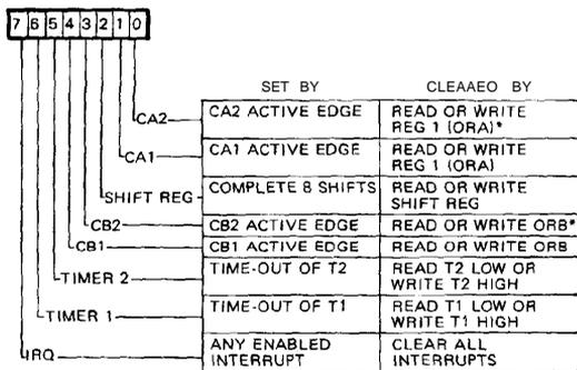
IF THE CA2/CB2 CONTROL IN THE PCR IS SELECTED AS "INDEPENDENT" INTERRUPT INPUT, THEN READING OR WRITING THE OUTPUT REGISTER ORA/ORB WILL NOT CLEAR THE FLAG BIT. INSTEAD, THE BIT MUST BE CLEARED BY WRITING INTO THE IFR, AS DESCRIBED PREVIOUSLY.
