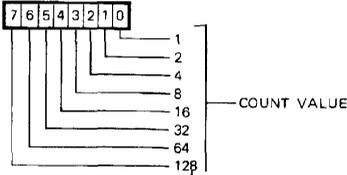
WRITE - 8 BITS ARE LOADED INTO T1 LOW-ORDER LATCHES. LATCH CONTENTS ARE TRANSFERRED INTO LOW ORDER COUNTER AT THE TIME THE HIGH ORDER COUNTER IS LOADED (REG. 5).
