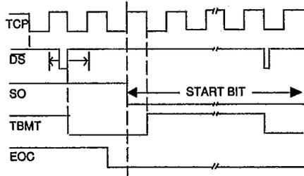
**FIG. 3 TRANSMITTER AT START BIT**
