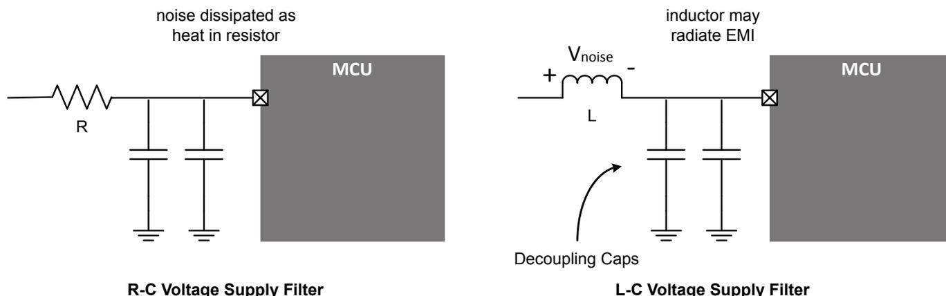
**Figure 1.3. Voltage Supply Filter Examples**
