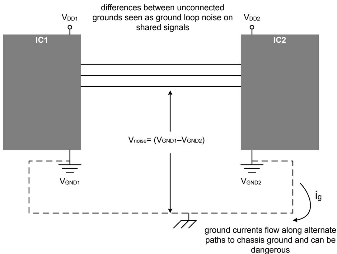
Figure 10.2. Ground Loop Created by Multiple Ground Connections
