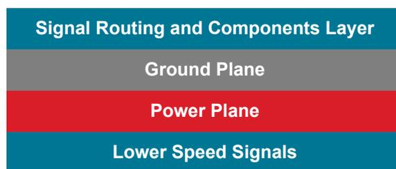
Figure 5.1. Four-Layer Board
