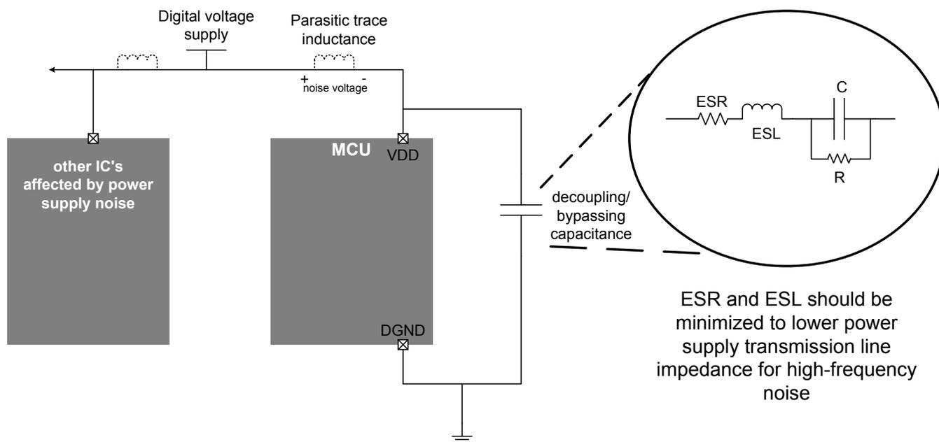
ESR and ESL should be minimized to lower power supply transmission line impedance for high-frequency noise
