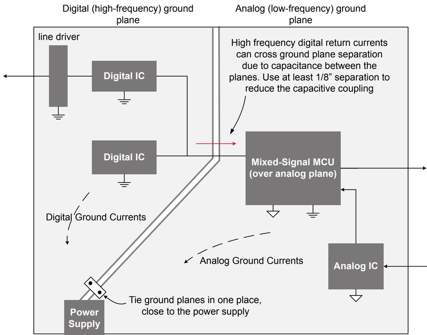
**Figure 1.6. Using Split Analog and Digital Ground Planes**
