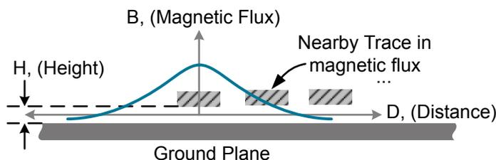
Figure 8.1. Magnetic Flux as a Function of Distance from a Trace
