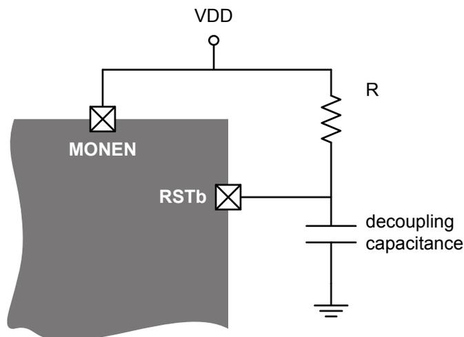
Figure 3.1. Decouple and Pull-Ups on the RSTb and MONEN Pins
