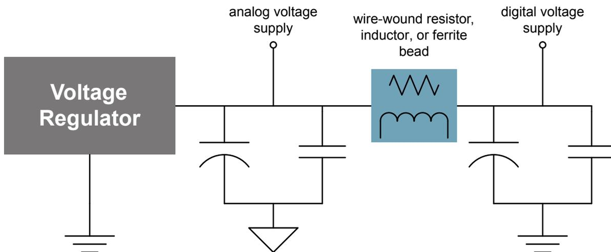
Figure 1.5. Filtering Analog Power Supply
