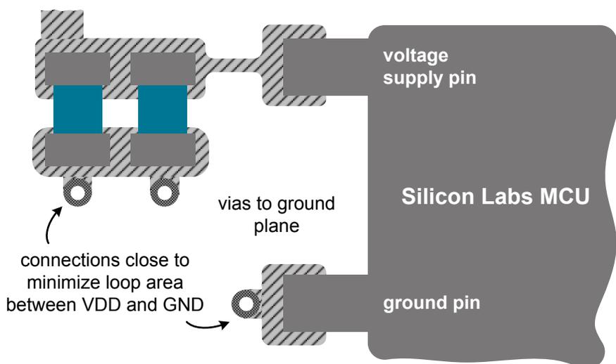
**Figure 1.4. Minimize Loop Area between Power and Ground**
