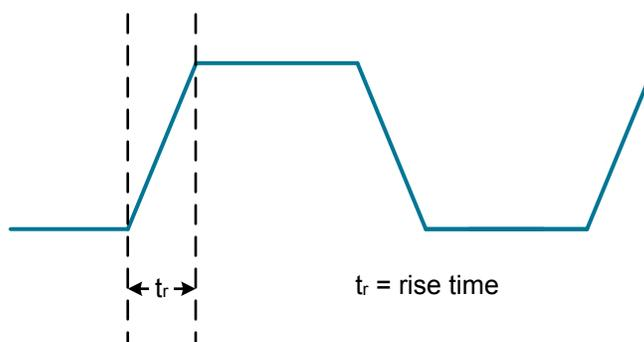
Figure 7.1. Digital Waveform Rise Time
