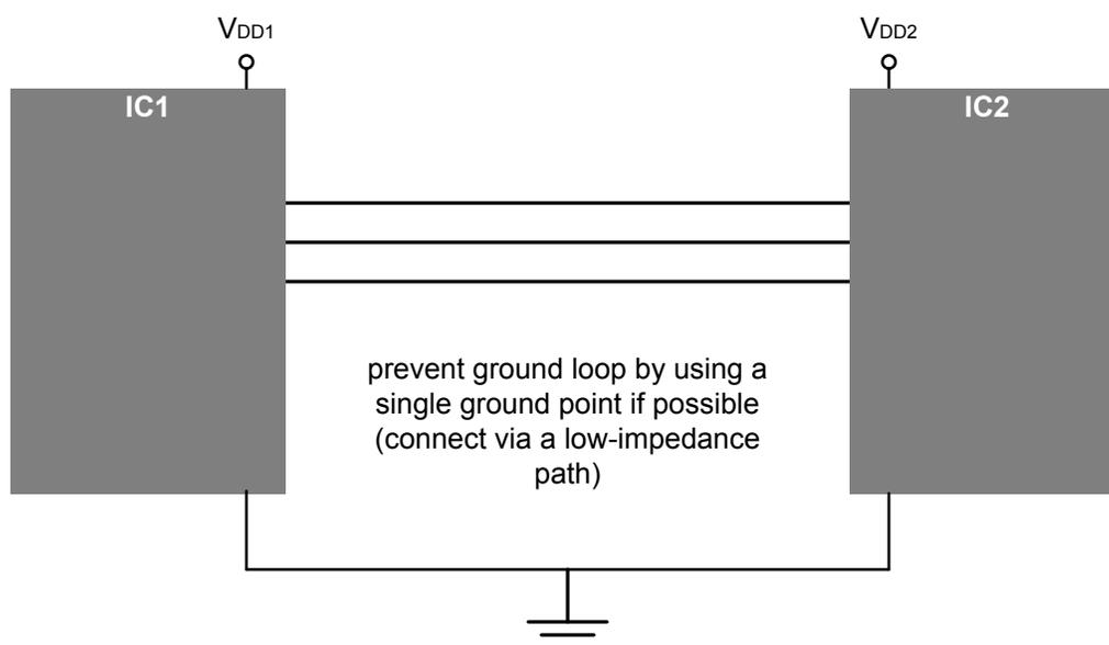
**Figure 10.4. Preventing Ground Loops by Sharing a Common Ground**
