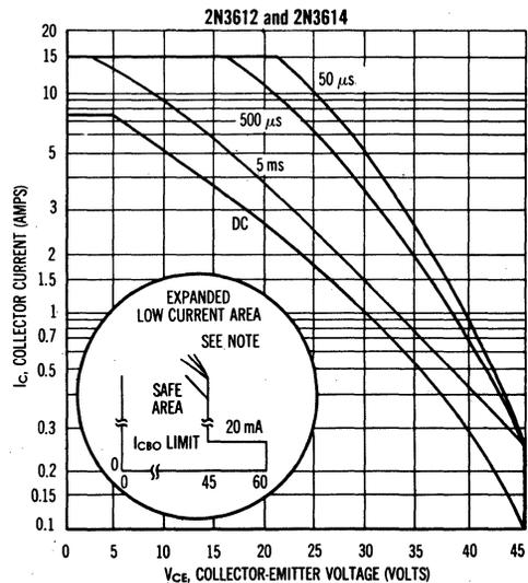
The Safe Operating Area Curves indicate  $I_C$ - $V_{CE}$  limits below which the device will not go into secondary breakdown. Collector load lines for specific circuits must fall within the applicable Safe Area to avoid causing a collector-emitter short. (Case temperature and duty cycle of the excursions make no significant change in these safe areas.) The load line may exceed the  $BV_{CES}$  voltage limit only if the collector
