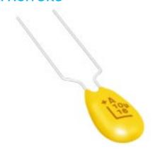
TAP is a professional grade device manufactured with a flame retardant coating and featuring low leakage current and impedance, very small physical sizes and exceptional temperature stability. It is designed and conditioned to operate to +125°C (see page 27 for voltage derating above 85°C) and is available loose or taped and reeled for auto insertion. The 15 case sizes with wide capacitance and working voltage ranges means the TAP can accommodate almost any application.
