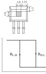
Applying direction of magnetic flux
