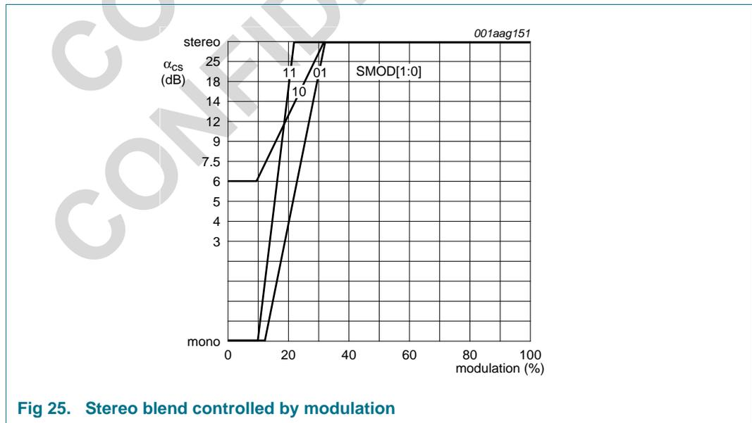
Fig 25. Stereo blend controlled by modulation
