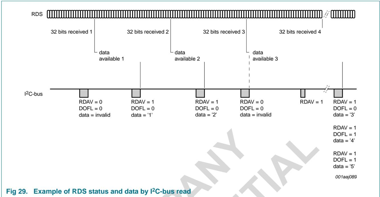
Fig 29. Example of RDS status and data by I2C-bus read
