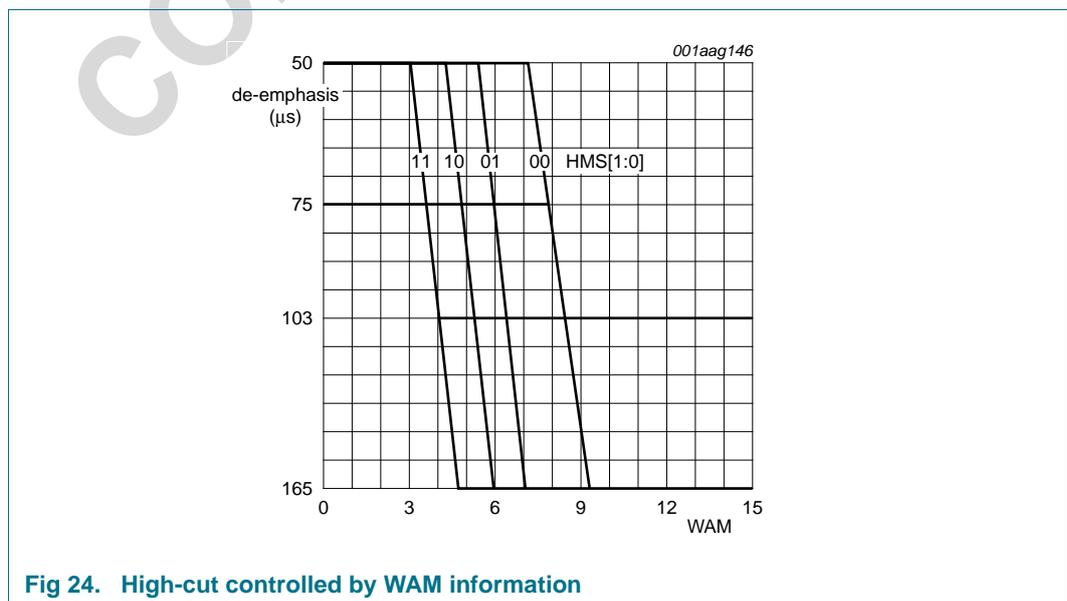
Fig 24. High-cut controlled by WAM information
