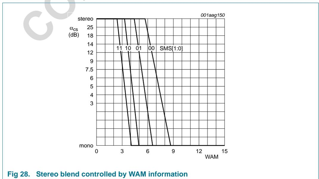
Fig 28. Stereo blend controlled by WAM information
