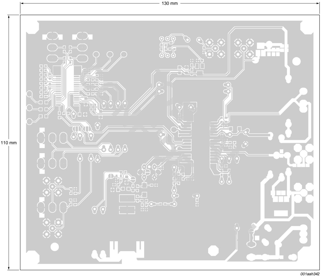
**Fig 31.** Printed-circuit board layout, suggested for application (this layout has been used in the NXP GH989 reference design, 35  $\mu\text{m}$ )
