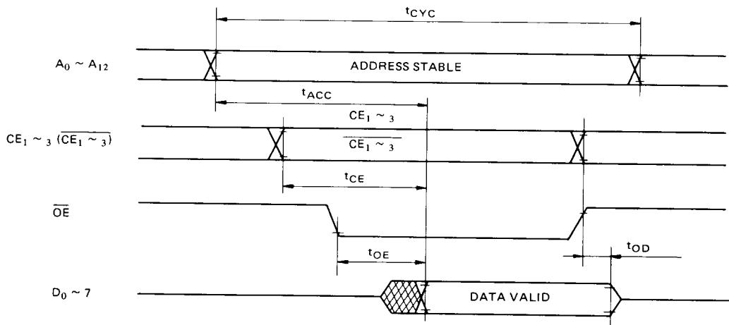
Note:  $t_{OD}$  is specified from  $\overline{OE}$  or  $CE/\overline{CE}$ , whichever occurs first.
