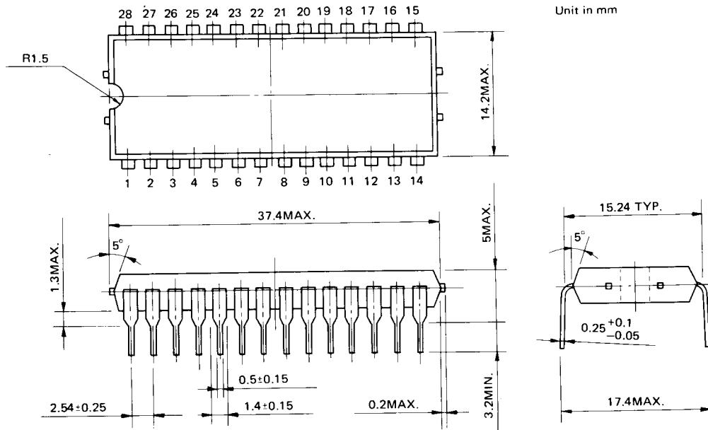
Note : Each lead pitch is 2.54mm. All leads are located within 0.25mm of their true longitudinal position with respect to No.1 and No.28 leads.
