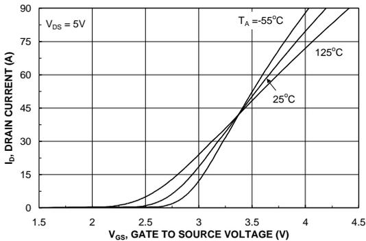
Figure 5. Transfer Characteristics
