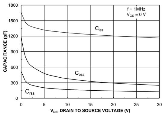
Figure 8. Capacitance Characteristics
