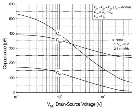
**Figure 5. Capacitance Characteristics**
