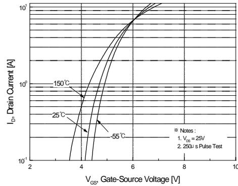
**Figure 2. Transfer Characteristics**
