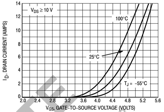
Figure 2. Transfer Characteristics
