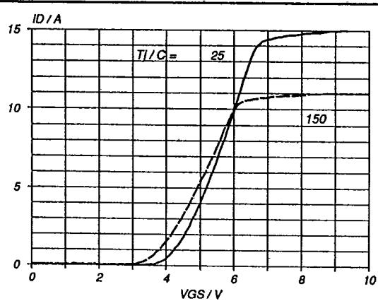
Fig. 8. Typical transfer characteristics.
