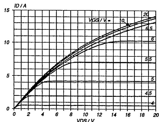
Fig. 6.<sup>1</sup> Typical output characteristics,  $T_j = 25^\circ\text{C}$ .
