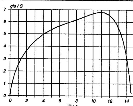
Fig. 9. Typical transconductance,  $T_j = 25^\circ\text{C}$ .
