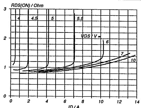
Fig. 7. Typical on-state resistance,  $T_j = 25^\circ\text{C}$ .
