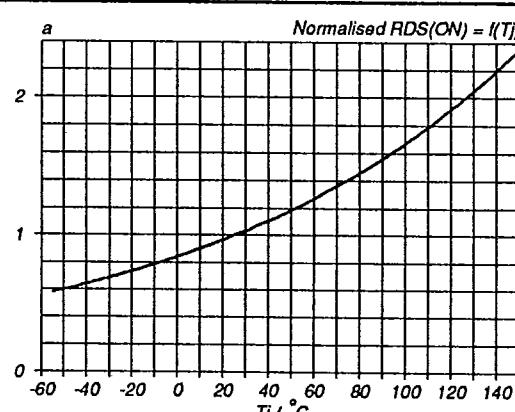
Fig. 10. Normalised drain-source on-state resistance.
