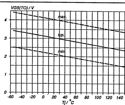
Fig. 11. Gate threshold voltage.
