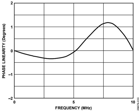
Figure 10. Phase Linearity Error in Minimal Configuration
