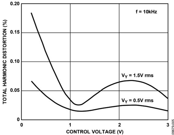
Figure 5. Total Harmonic Distortion vs. Control Voltage
