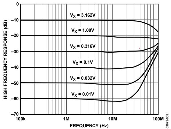
Figure 9. High Frequency Response in Minimal Configuration
