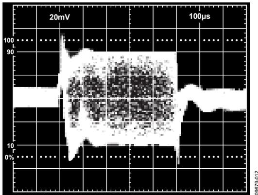
Figure 12. Control Feedthrough One Channel of Figure 22
