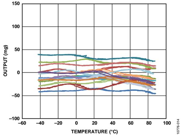
Figure 14. X-Axis Zero g Offset vs. Temperature—
