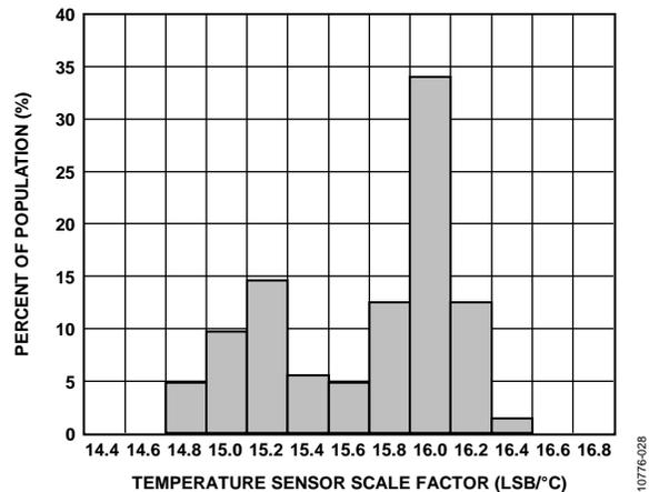
Figure 28. Temperature Sensor Scale Factor,  $V_S = 2 V$
