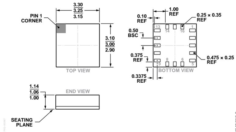
Figure 53. 16-Terminal Land Grid Array [LGA]
