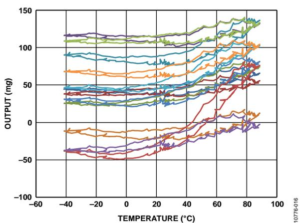
Figure 16. Z-Axis Zero g Offset vs. Temperature—
