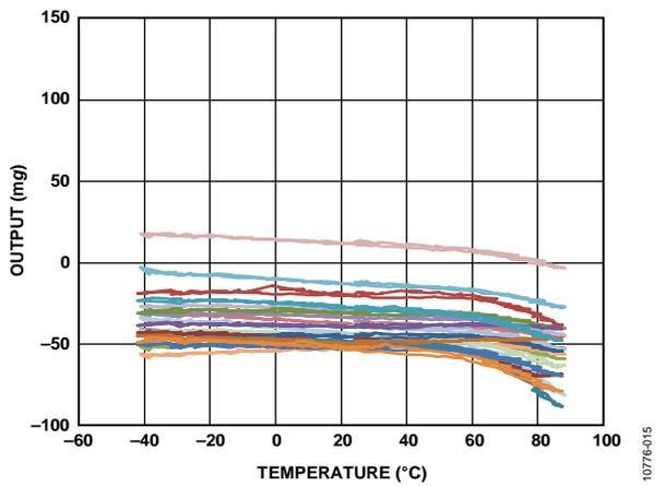
Figure 15. Y-Axis Zero g Offset vs. Temperature—
