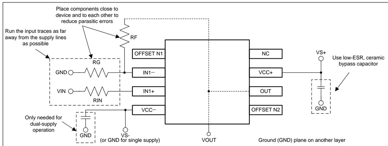
**Figure 18. Operational Amplifier Board Layout for Noninverting Configuration**
