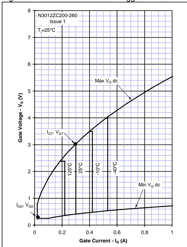
Figure 4 - Gate characteristics - Power curves
