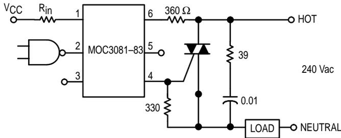
Typical circuit for use when hot line switching is required. In this circuit the "hot" side of the line is switched and the load connected to the cold or neutral side. The load may be connected to either the neutral or hot line.
