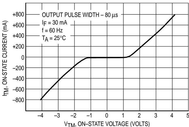
Figure 1. On-State Characteristics
