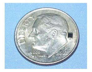
NoiseWave announces the immediate availability of the NW301 surface mount noise diode. The unit features broadband frequency coverage from 10 MHz to 3.5 GHz. Output ENR is 32 dB minimum with greater than 35 dB typical. The diode voltage range is 8-12 V and the current is specified at 5 mA however it can be run at different currents depending on the application.
