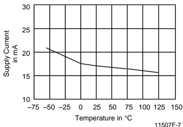
**Figure 2. Typical Supply Current vs. Temperature**
