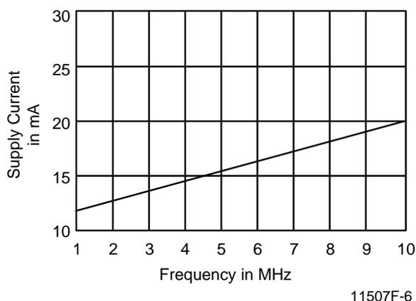
**Figure 1. Typical Supply Current vs. Frequency**
