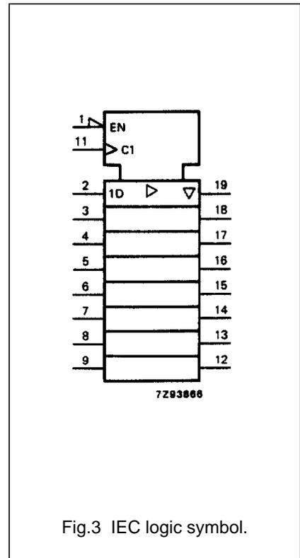
Octal D-type flip-flop; positive edge-trigger;
