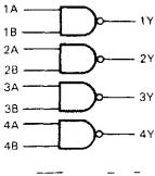
$Y = \overline{A \cdot B}$  or  $Y = \overline{A} + \overline{B}$
