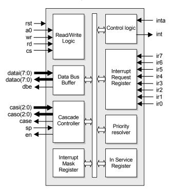
Cascade Controller - The Cascade Controller stores and compares Identifiers of all 8259 devices in the system. Block manages direction of CAS input/output buses, depending of device status: Master or Slave. When operating as a master the D8259 drives onto the CAS bus address of interrupting 8259 device, then the addressed 8259 slave during the next one or two consecutive INTA pulses send to the Data Bus preprogrammed address of subroutine.
