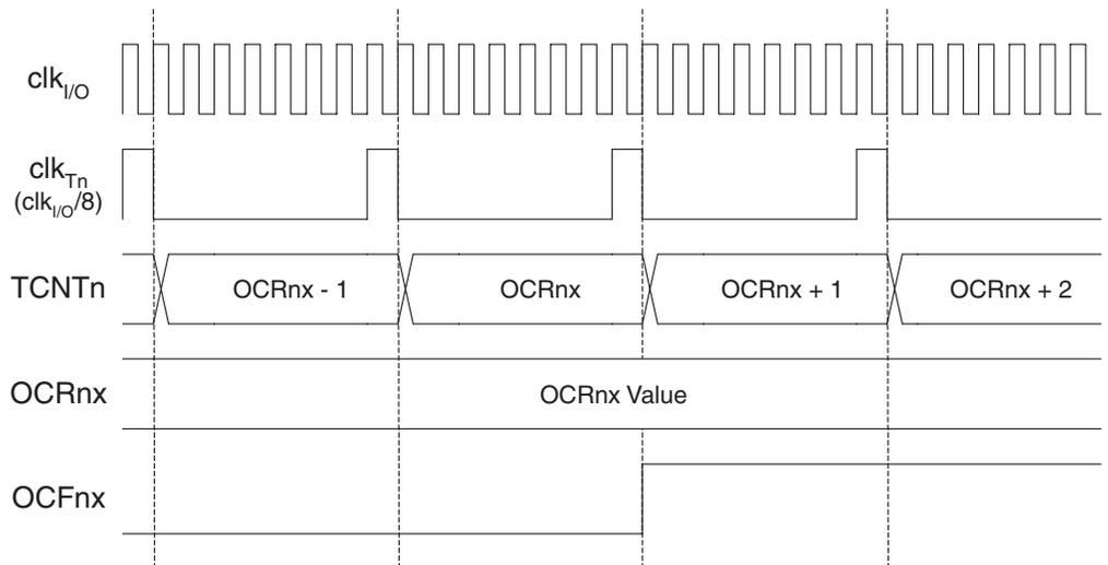
Figure 51 shows the count sequence close to TOP in various modes. When using phase and frequency correct PWM mode the OCR1x Register is updated at BOTTOM. The timing diagrams will be the same, but TOP should be replaced by BOTTOM, TOP-1 by BOTTOM+1 and so on. The same renaming applies for modes that set the TOV1 flag at BOTTOM.
