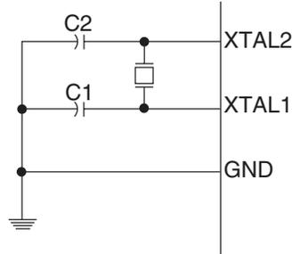
The Oscillator can operate in three different modes, each optimized for a specific frequency range. The operating mode is selected by the fuses CKSEL3..1 as shown in Table 4.
