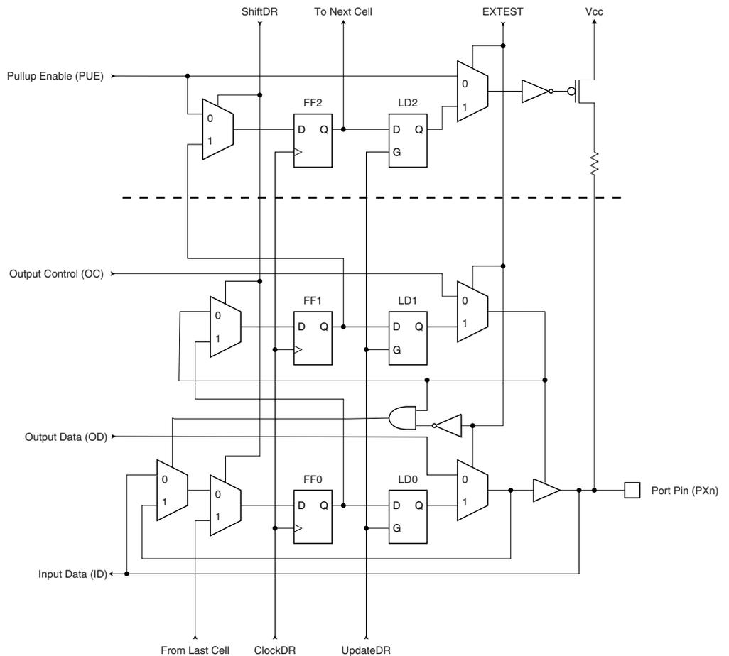
**Figure 117. General Port Pin Schematic Diagram<sup>(1)</sup>**
