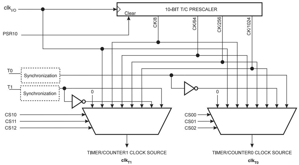
Note: 1. The synchronization logic on the input pins (T1/T0) is shown in Figure 38.
