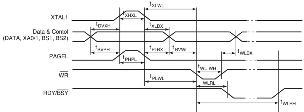
**Figure 134.** Parallel Programming Timing, Loading Sequence with Timing Requirements<sup>(1)</sup>
