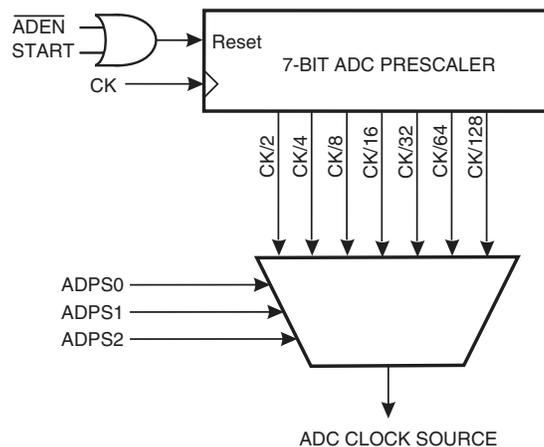
By default, the successive approximation circuitry requires an input clock frequency between 50 kHz and 200 kHz to get maximum resolution. If a lower resolution than 10 bits is needed, the input clock frequency to the ADC can be higher than 200 kHz to get a higher sample rate. Alternatively, setting the ADHSM bit in SFIOR allows an increased ADC clock frequency at the expense of higher power consumption.
