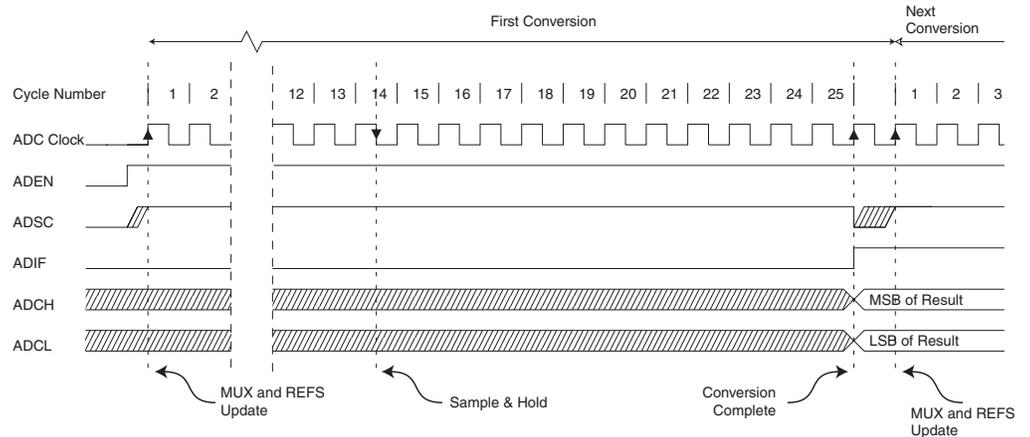
**Figure 102. ADC Timing Diagram, Single Conversion**
