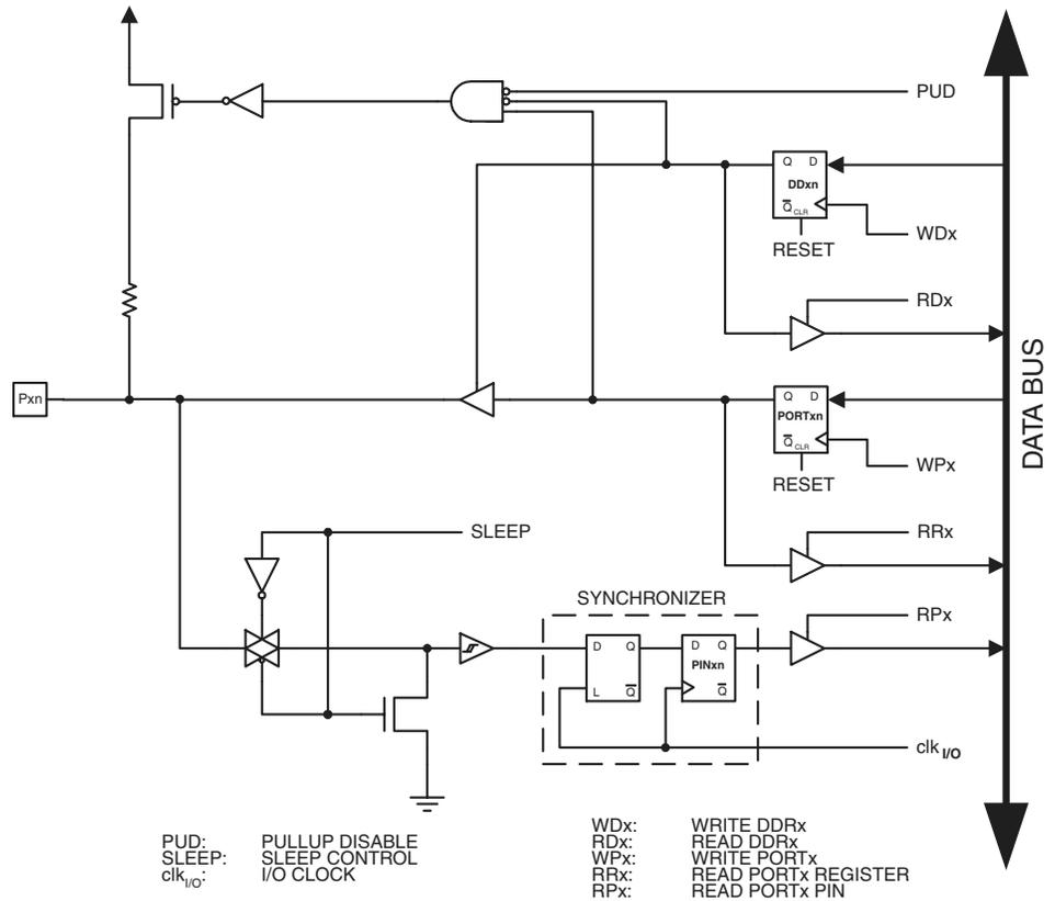
Note: 1. WP<sub>x</sub>, WD<sub>x</sub>, RR<sub>x</sub>, RP<sub>x</sub>, and RD<sub>x</sub> are common to all pins within the same port. clk<sub>I/O</sub>, SLEEP, and PUD are common to all ports.
