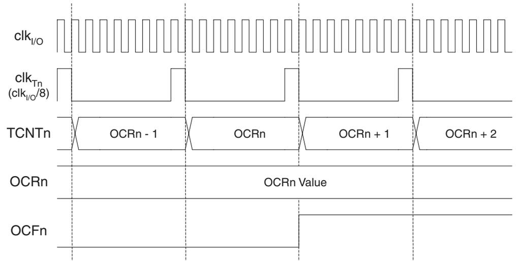
Figure 37 shows the setting of OCF0 and the clearing of TCNT0 in CTC mode.
