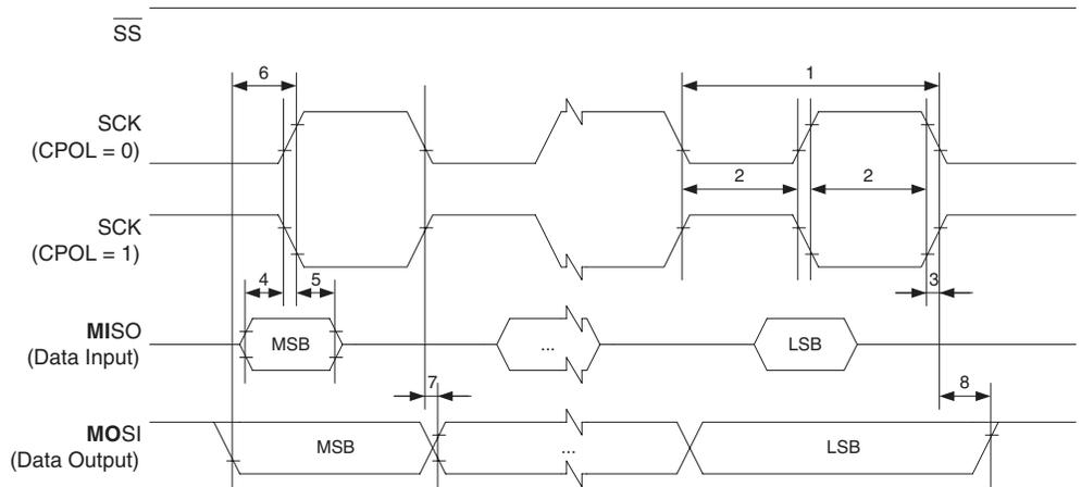
**Figure 147. SPI Interface Timing Requirements (Slave Mode)**
