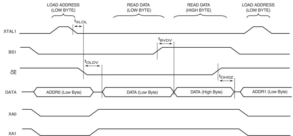
Note: 1. The timing requirements shown in Figure 133 (i.e.,  $t_{DVXH}$ ,  $t_{XHXL}$ , and  $t_{XLDX}$ ) also apply to reading operation.
