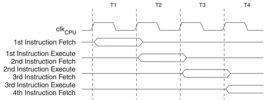
Figure 7 shows the internal timing concept for the Register file. In a single clock cycle an ALU operation using two register operands is executed, and the result is stored back to the destination register.
