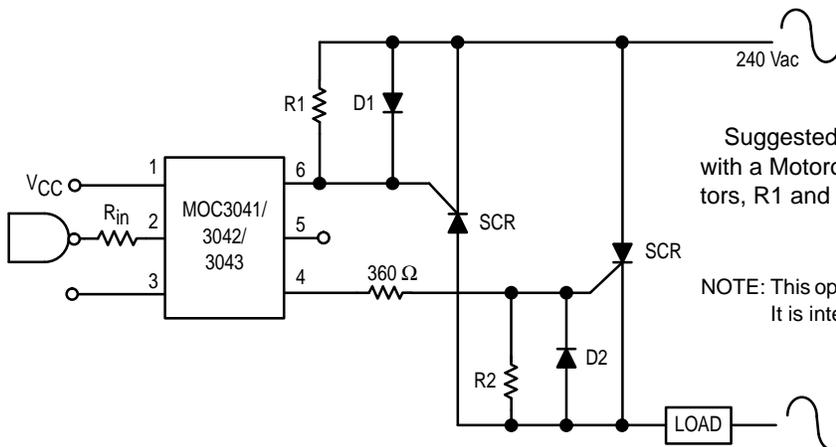
Suggested method of firing two, back-to-back SCR's, with a Motorola triac driver. Diodes can be 1N4001; resistors, R1 and R2, are optional 330 ohms.
