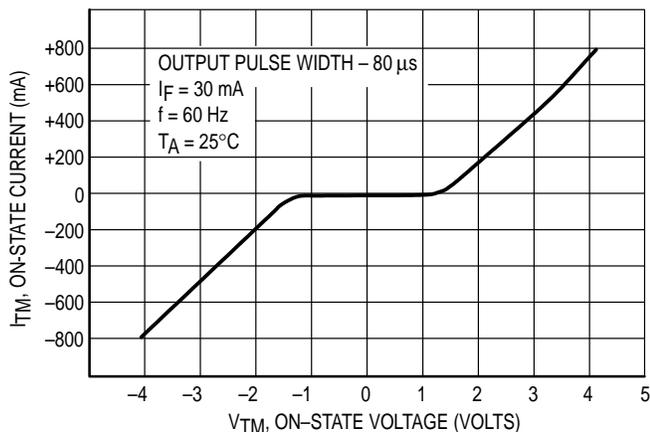
**Figure 1. On-State Characteristics**
