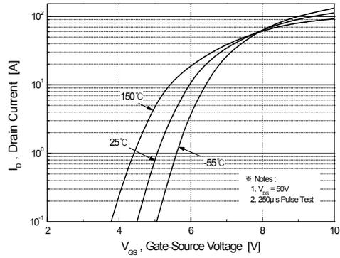
**Figure 2. Transfer Characteristics**
