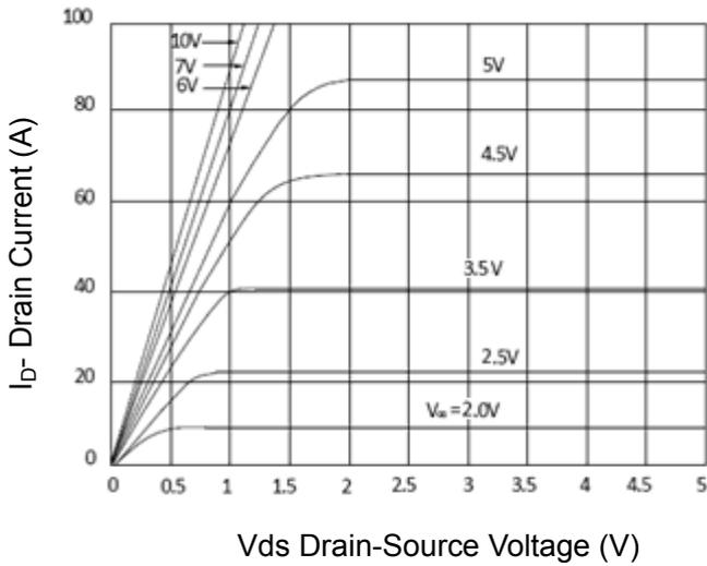
Figure 1 Output Characteristics
