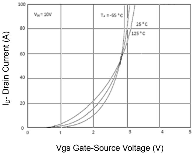
Figure 2 Transfer Characteristics
