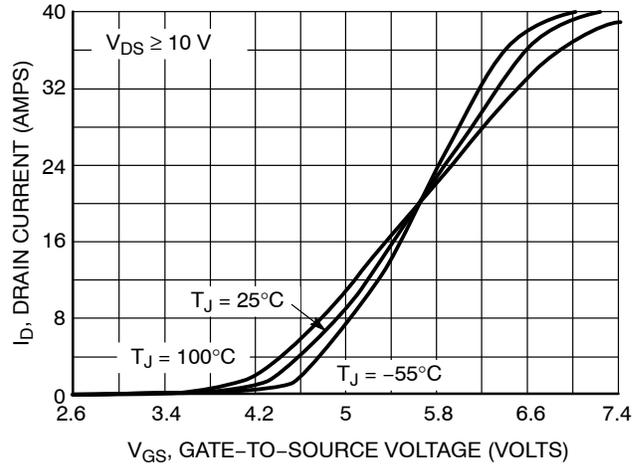
Figure 2. Transfer Characteristics
