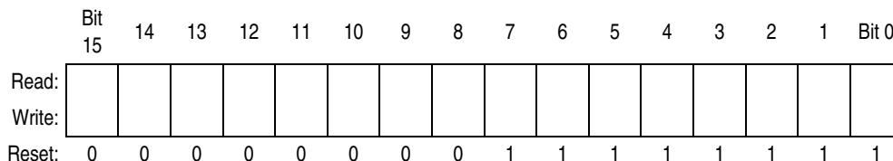
Figure 4-4. Stack Pointer (SP)
