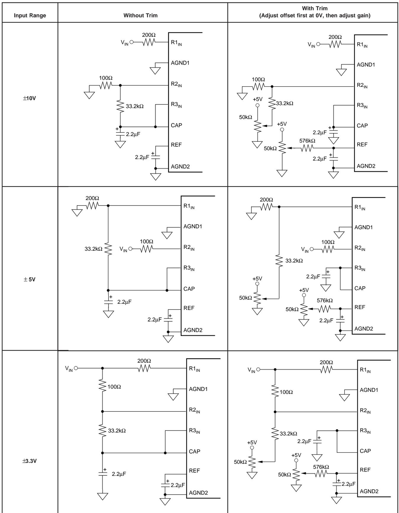
FIGURE 4b. Offset/Gain Circuits for Bipolar Input Ranges.
