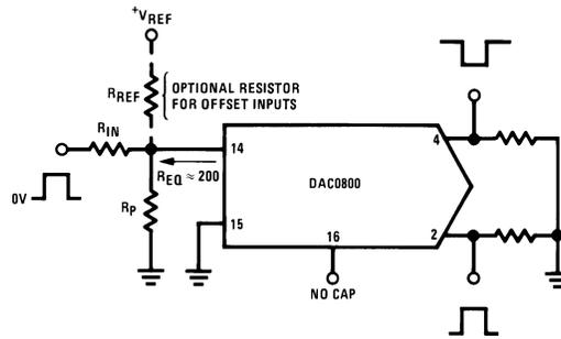
Typical values:  $R_{IN}=5k, +V_{IN}=10V$
