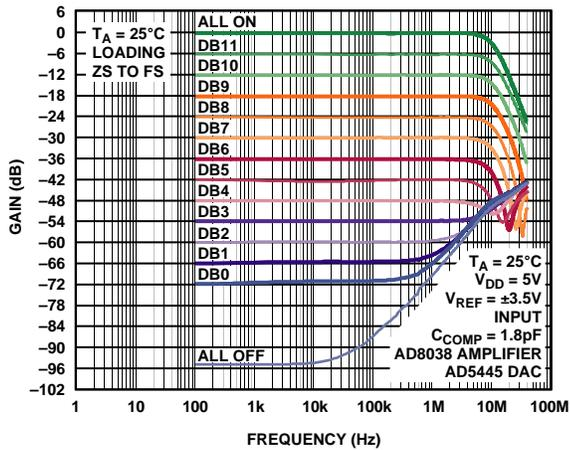
Figure 28. Reference Multiplying Bandwidth vs. Frequency and Code
