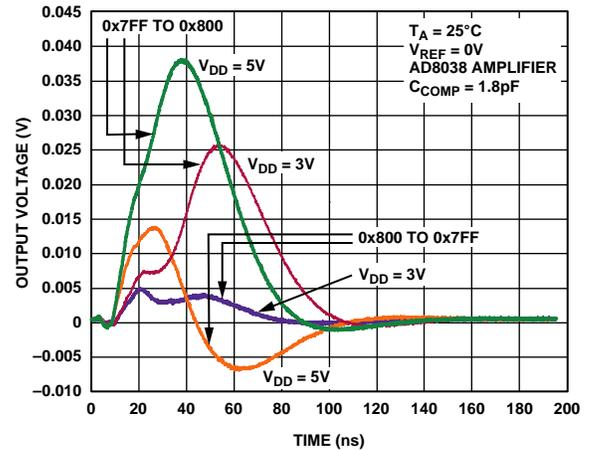
Figure 31. Midscale Transition,  $V_{REF} = 0\text{ V}$
