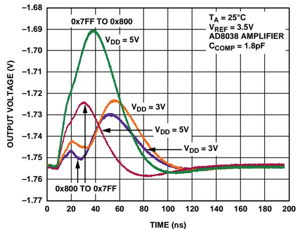
Figure 32. Midscale Transition,  $V_{REF} = 3.5\text{ V}$
