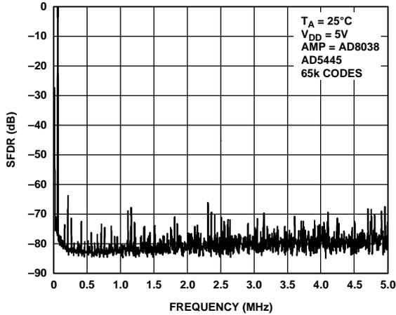
Figure 40. Wideband SFDR,  $f_{OUT} = 50$  kHz, Clock = 10 MHz
