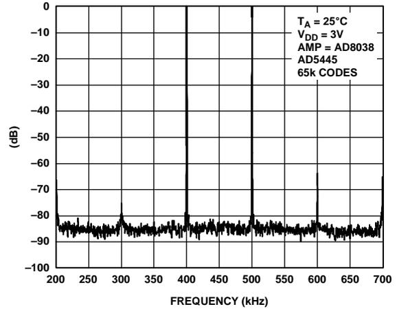
Figure 43. Narrow-Band IMD,  $f_{OUT} = 400$  kHz, 500 kHz, Clock = 10 MHz
