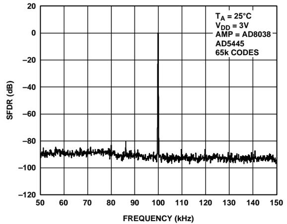
Figure 42. Narrow-Band SFDR,  $f_{OUT} = 100$  kHz, MCLK = 25 MHz
