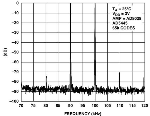
Figure 44. Narrow-Band IMD,  $f_{OUT} = 90$  kHz, 100 kHz, Clock = 10 MHz
