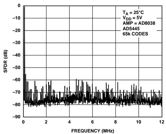
Figure 38. Wideband SFDR,  $f_{OUT} = 100\text{ kHz}$ , Clock = 25 MHz
