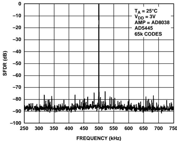
Figure 41. Narrow-Band Spectral Response,  $f_{OUT} = 500$  kHz, Clock = 25 MHz
