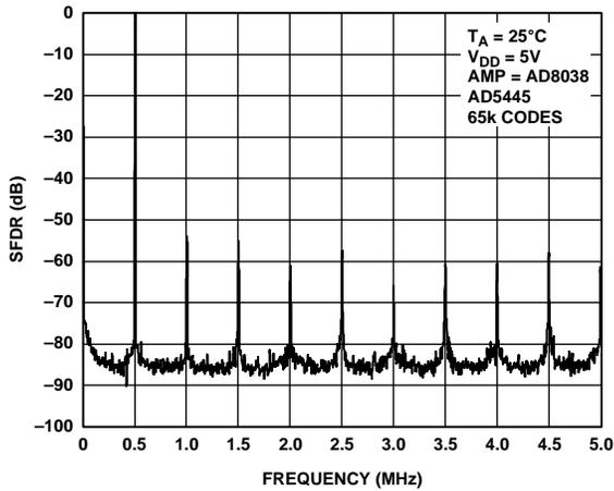
Figure 39. Wideband SFDR,  $f_{OUT} = 500$  kHz, Clock = 10 MHz
