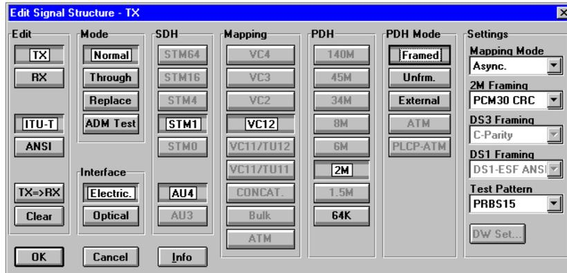
Fig. VI-2 Displaying and setting the signal structure using ITU-T (Tx side) as an example
