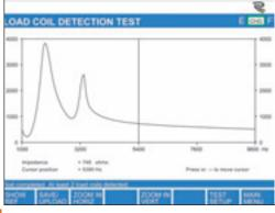
Easilty Detect Number of Load Coils Deployed
