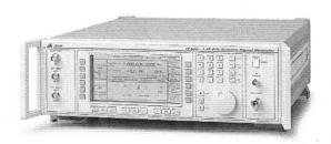
Ability to offset for insertion loss or gain of external devices, and provides complex carrier sweeps. Particularly useful for EMC testing and for ATE applications.
