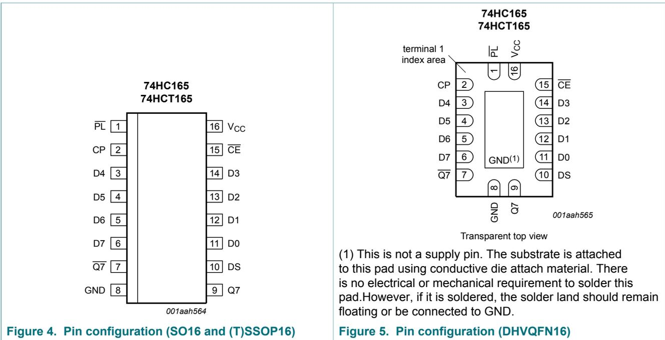
Figure 4. Pin configuration (SO16 and (T)SSOP16)
