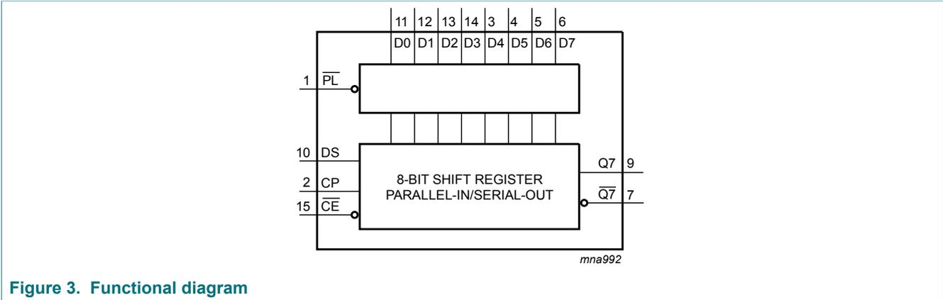
Figure 3. Functional diagram
