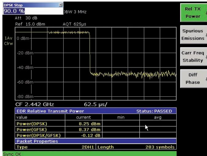
All measurements are carried out in line with the Bluetooth® RF Test Specification (Bluetooth® SIG) Rev. 2.0+EDR and cover basic rate as well as EDR. Integrated limit value monitoring is provided for all measurements and allows analysis of the results in the development and production of Bluetooth® modules.
