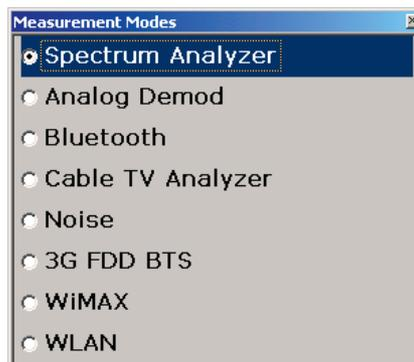
The R&S®FSL offers many different firmware options (see page 22). The user can switch between the different applications.
