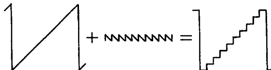
Figure 3.10 Representation of the discrete modulating function by the sum of two sawtooth functions.
