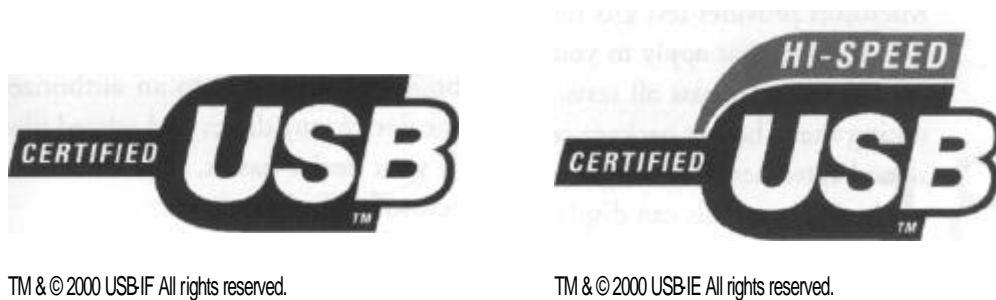
Figure 17-10: Devices that pass compliance testing can display the USB Logo. The logo indicates if the device supports high speed.
