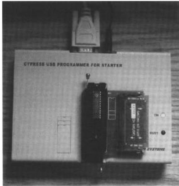
Figure 9-4: Cypress offers an inexpensive programmer and adapters for the enCoRe series and other chips. The photo shows an Adapter Base inserted into the programmer's ZIP socket. The Adapter Base holds a matrix card and a chip to be programmed.
