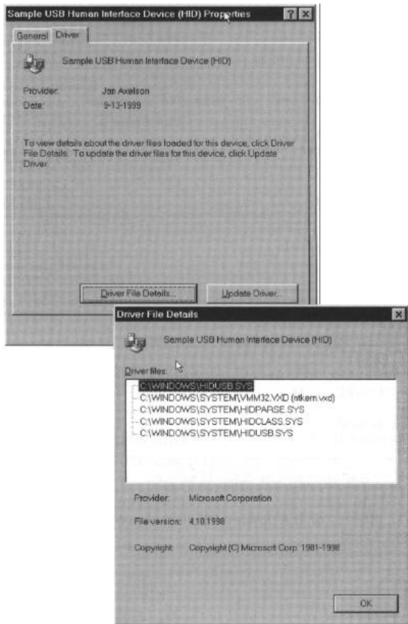
Figure 11-5: The information displayed by the Device Manager includes the Provider name and drivers specified in the device's INF file.
