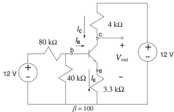
5. In the following circuit find  $R_1$ ,  $R_2$ ,  $R_E$ , and  $R_C$  such that  $I_E = 1 \text{ mA}$ ,  $V_{cd} = 3.3 \text{ V}$ ,  $V_{bd} = 4 \text{ V}$ , and  $V_{cd} = 8 \text{ V}$ .
