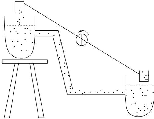
**FIGURE 2.4:** A water circuit.
