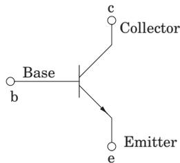
**FIGURE 6.1:** A bipolar junction transistor.
