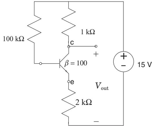
11. In the circuit below find  $I_c$  and  $V_{ce}$ .
