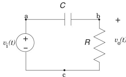
**FIGURE 4.12:** High pass filter.
