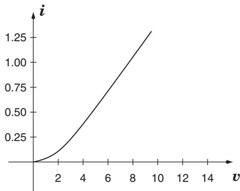
**FIGURE 5.16:** Nonlinear component rule.
