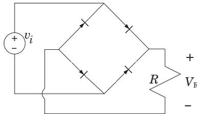
2. In the circuits shown below what is the value of  $V_{\text{out}}$  if (i)  $V_{\text{in}} = 15 \text{ V}$  and (ii)  $V_{\text{in}} = -5 \text{ V}$ ? Assume  $V_T = 0.7 \text{ V}$ .
