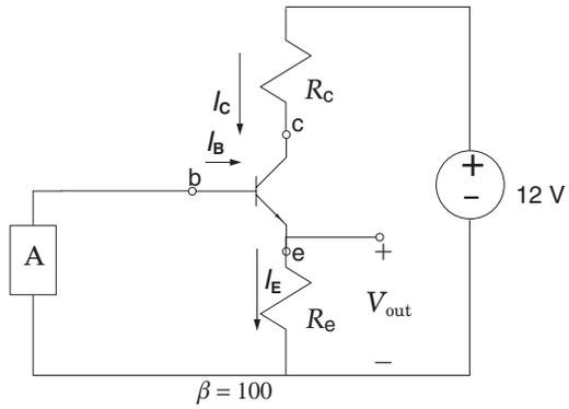
8. In the following circuit find  $I_c$  and  $V_{out}$ .
