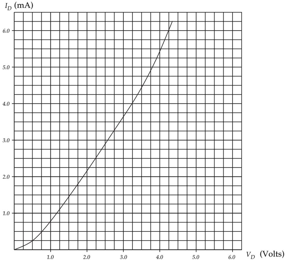
**FIGURE 5.21:** Diode component rule.
