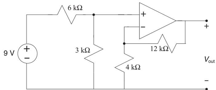
5. In the following circuit find  $V_{out}$ .
