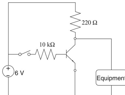
**FIGURE 6.15:** A normally on switch.
