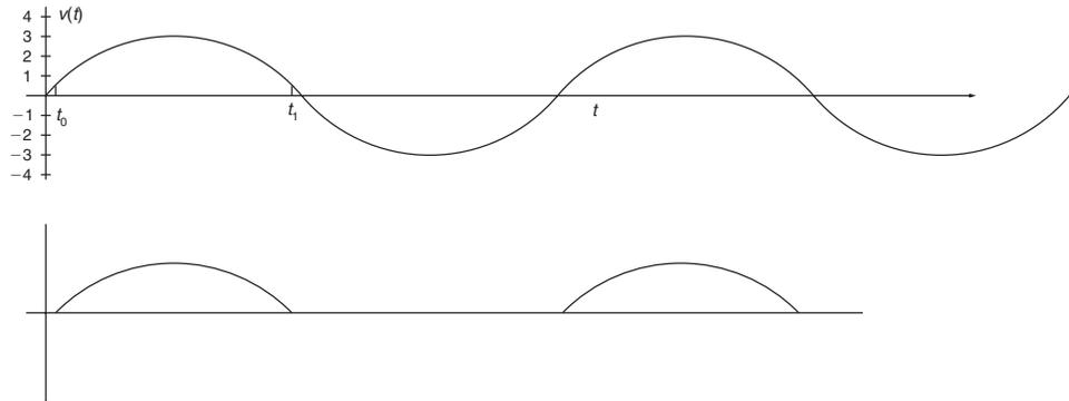
**FIGURE 5.6:** Input and output of half-wave rectifier.
