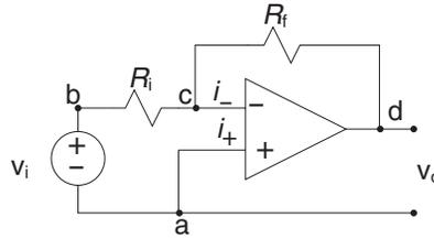
**FIGURE 7.7:** A simple op-amp circuit.
