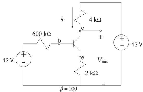
4. In the circuit shown below find  $I_C$ ,  $I_B$ ,  $I_E$ , and  $V_{out}$ .
