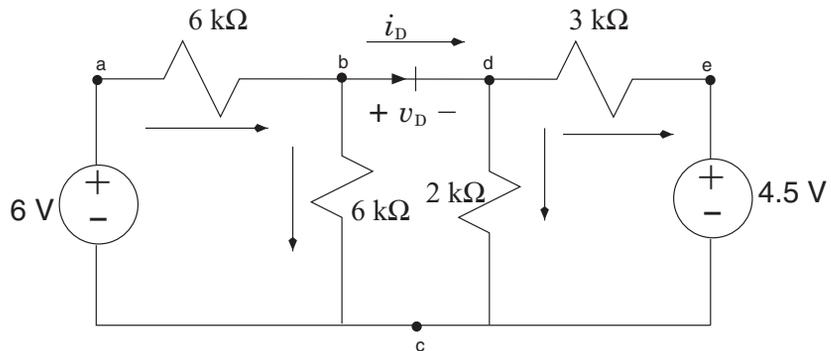
**FIGURE 5.20:** Diode circuit.
