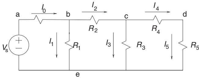
**FIGURE 3.5:** An example of a resistive circuit.
