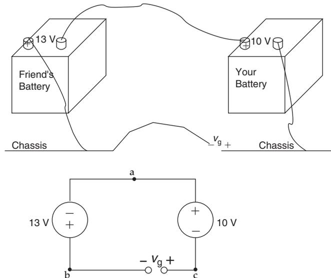
**FIGURE 2.17:** Incorrect way to connect batteries.
