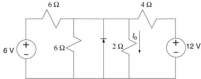
5. In the following circuit find  $I_o$ . Assume an ideal diode with a threshold voltage of 0.7 V. *Justify all assumptions.*
