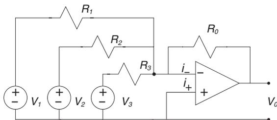
**FIGURE 7.9:** A summing amplifier circuit.
