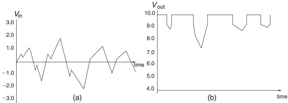
**FIGURE 6.5:** Clipping during amplification.
