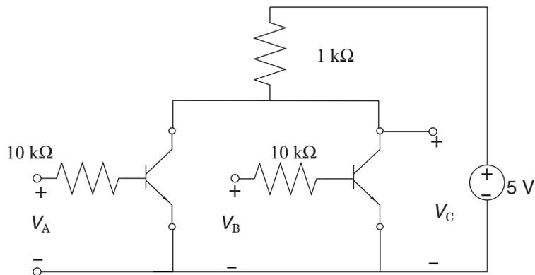
**FIGURE 6.13:** A two input NOR gate.
