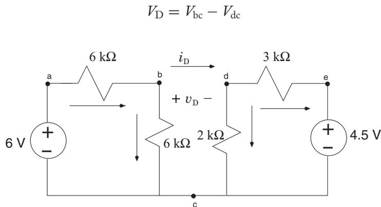
**FIGURE 5.23:** Circuit to find the  $x$ -axis intercept.
