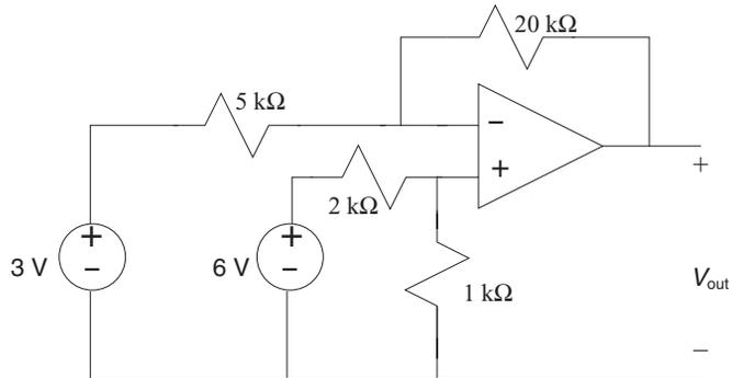
8. In the following circuit find  $V_{out}$  when  $V_{in} = 0.5$  V.
