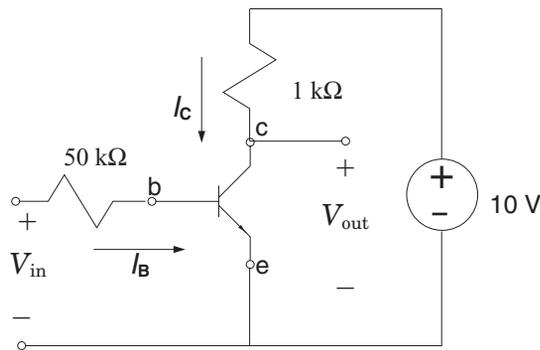
2. For the circuit shown below find  $I_c$  and  $V_{out}$  for  $V_{in} = 2\text{ V}, 3\text{ V}, 4\text{ V}, 5\text{ V}, 6\text{ V}, 7\text{ V}, 8\text{ V}, 9\text{ V},$  and  $10\text{ V}$ . Present your answer in two ways: (a) Make a table with columns for  $V_{in}$ ,  $I_c$ , and  $V_{out}$ . (b) Plot  $V_{out}$  and  $I_c$  versus  $V_{in}$ .
