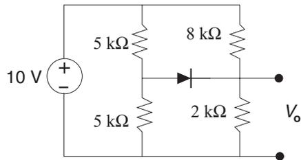
7. In the following circuit find  $V_o$ . Use the  $I$ - $V$  characteristic for the diode shown.
