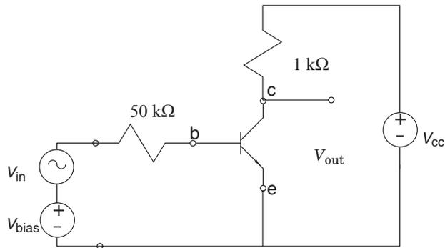
**FIGURE 6.7:** Transistor with amplifier.
