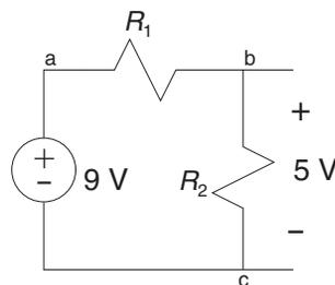
**FIGURE 3.9:** voltage divider.
