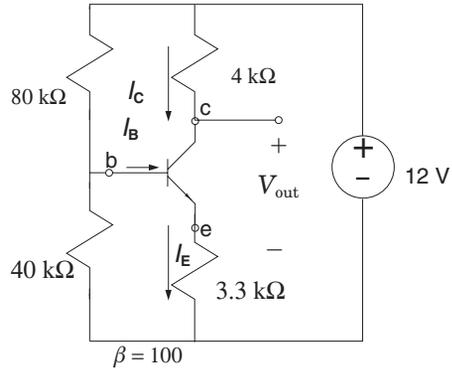
9. In the circuit shown below find  $I_c$  and  $V_{ce}$ .
