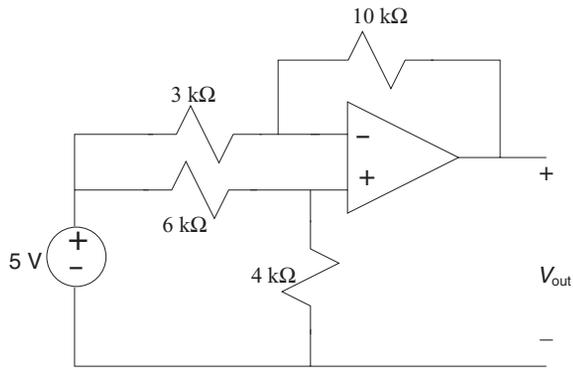
6. In the following circuit find  $V_{out}$ .
