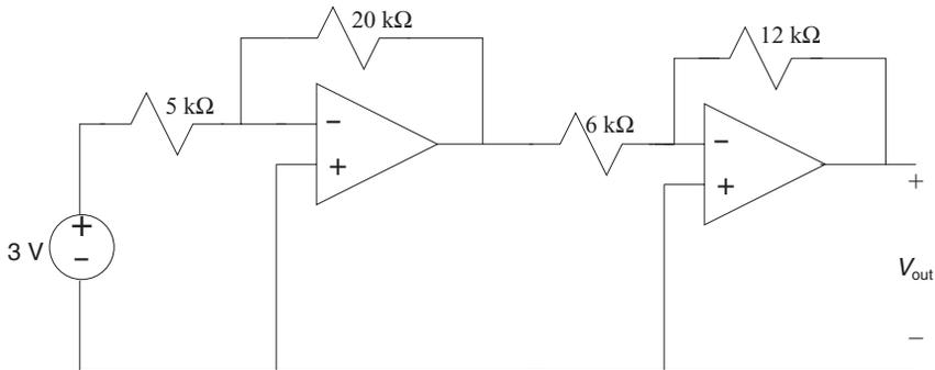
7. In the following circuit find  $V_{out}$ .
