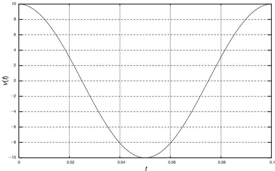
**FIGURE 4.4:** One cycle of sinusoid with frequency 10 Hz.
