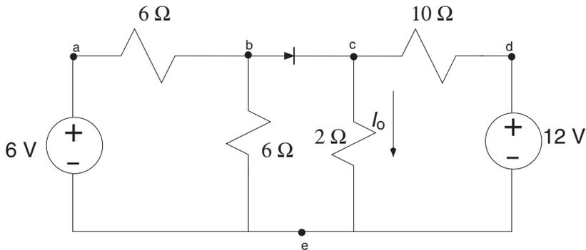
**FIGURE 5.13:** A circuit containing a diode.
