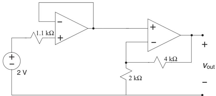
4. In the circuit below find  $V_{out}$ .
