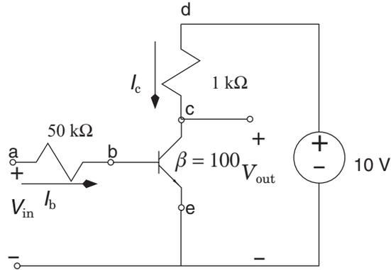
**FIGURE 6.2:** A common emitter amplifier.
