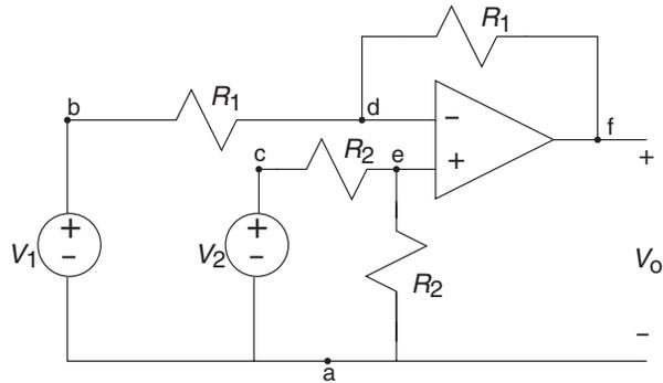
**FIGURE 7.10:** A difference circuit.
