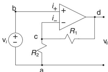
**FIGURE 7.8:** A noninverting amplifier circuit.
