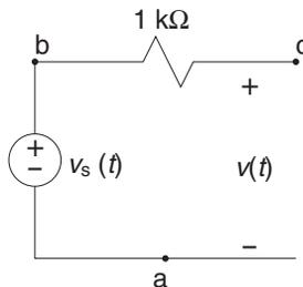
**FIGURE 4.8:** The open circuit approximation.
