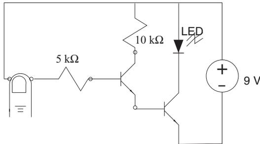
**FIGURE 6.10:** A touch-sensitive circuit.
