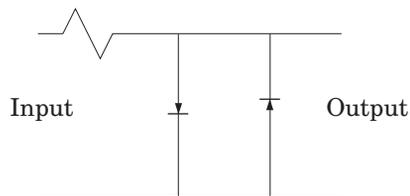
**FIGURE 5.12:** A limiting circuit.
