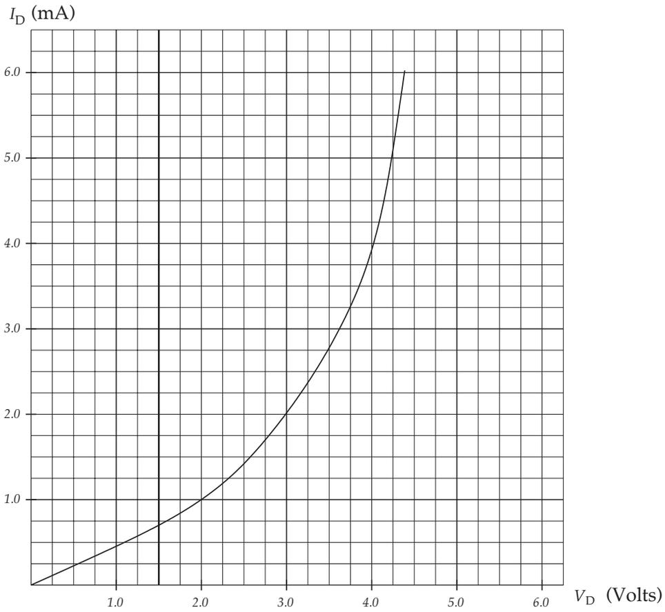
8. In the following circuit find  $I_o$ . Use the  $I$ - $V$  characteristic for the diode shown.
