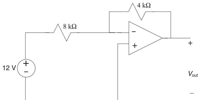
2. In the following circuit find  $V_{out}$ .
