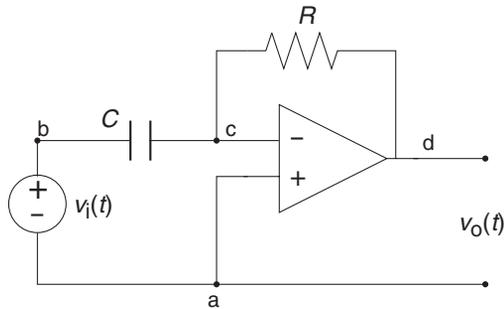
**FIGURE 7.13:** A differentiator circuit.
