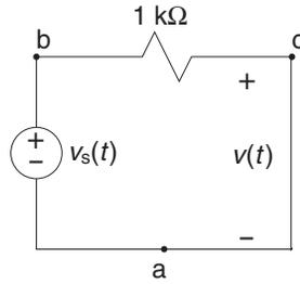
**FIGURE 4.9:** The short circuit approximation.
