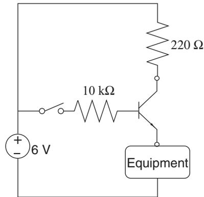
**FIGURE 6.14:** A normally off switch.
