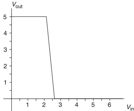
**FIGURE 6.12:** Input–output behavior of the NOT gate.
