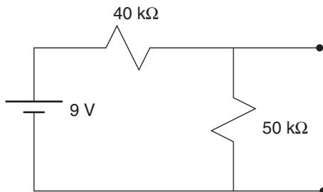
**FIGURE 7.4:** Voltage divider circuit.
