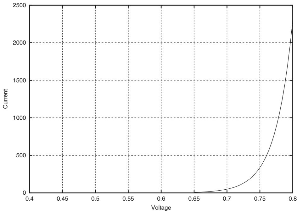
**FIGURE 5.2:** Current–voltage characteristic for a diode.
