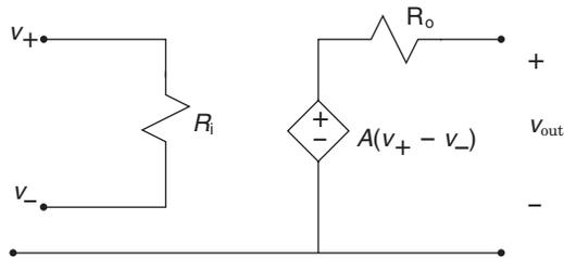
**FIGURE 7.2:** A model for an operational amplifier.
