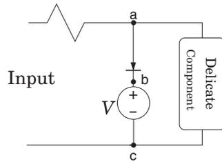
**FIGURE 5.11:** A diode clamp.
