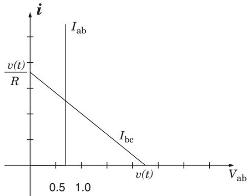
**FIGURE 5.19:** Graphical solution for ideal diode.
