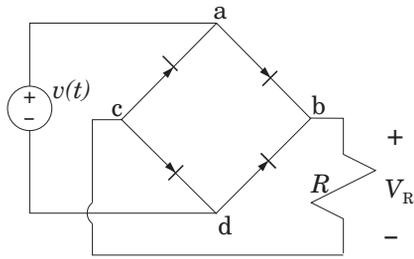
**FIGURE 5.7:** A full-wave rectifier.
