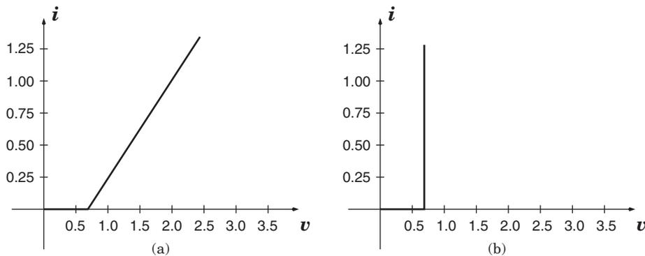
**FIGURE 5.3:** Approximations to the current–voltage characteristic for a diode.
