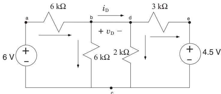
**FIGURE 5.24:** Circuit for finding the  $y$ -axis intercept.
