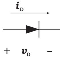
**FIGURE 5.1:** Symbol for diode.
