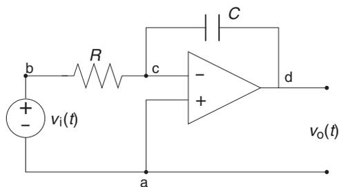
**FIGURE 7.12:** An integrator circuit.
