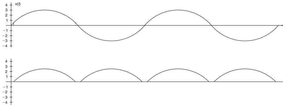
**FIGURE 5.10:** Input and output of a full-wave rectifier.
