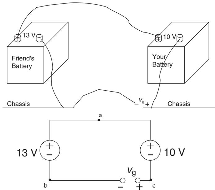
**FIGURE 2.16:** Correct way to connect the batteries.
