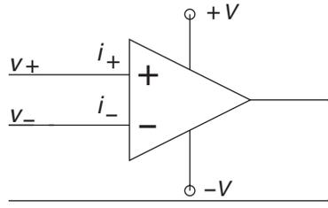
**FIGURE 7.1:** A symbol for an operational amplifier.
