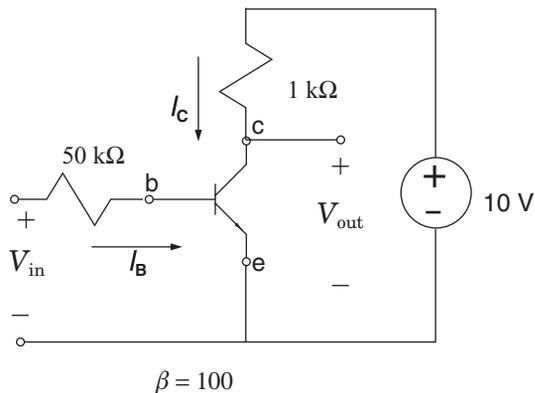
3. In the following circuit find  $I_C$  and  $V_{out}$ . You can assume that the transistor is not saturated (in other words you don't have to show that it is not saturated).
