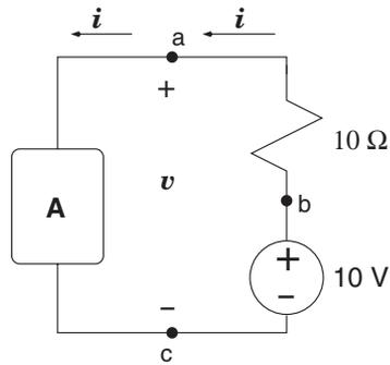
**FIGURE 5.15:** Circuit with nonlinear component.
