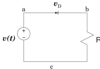
**FIGURE 5.4:** A simple diode circuit.
