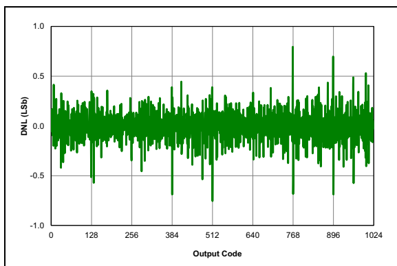
FIGURE 32-77: ADC 10-bit Mode, Single-Ended DNL, V_{DD} = 3.0V , T_{AD} = 1\ \mu S , 25^\circ C .
