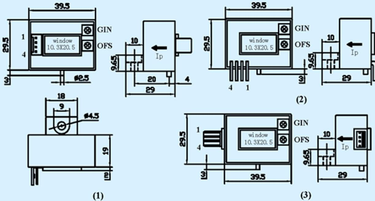
Elucidation: 1:+15V 2:-15V 3:V<sub>OUT</sub> 4:0V(GND) OFS:Zero adjustment GIN:Gain adjustment
